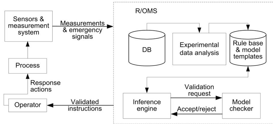
Figure 3.1 Model checking in an operator advisory system
