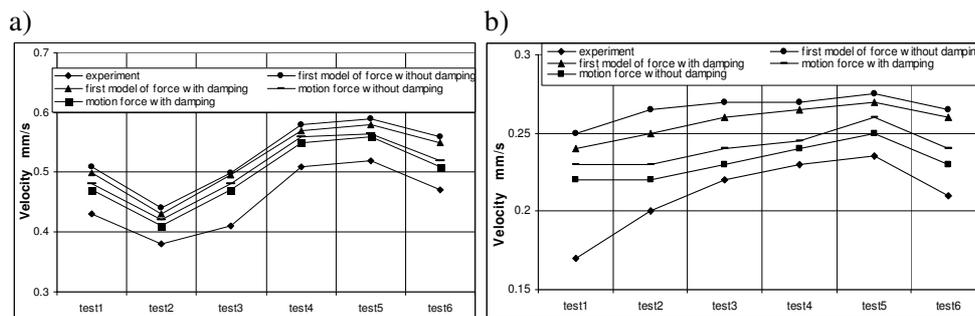
Figure 2.13 Comparative analysis of experimental and theoretical results (dynamical model with one degree of freedom) about horizontal (a) and vertical (b) vibrations by cutting
