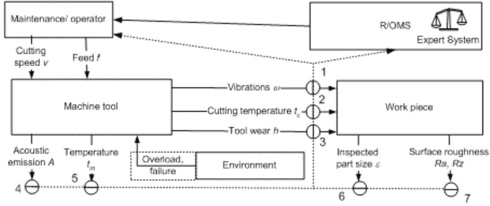
Fig. 3.2 Functional dependencies of IMM modules, where  $\textcircled{\mid}$  – monitored resettable variables of the model
