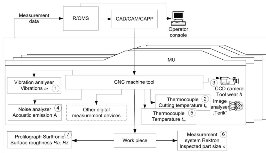
Figure 2.5 Planned data flows in the Intelligent Machining Unit
