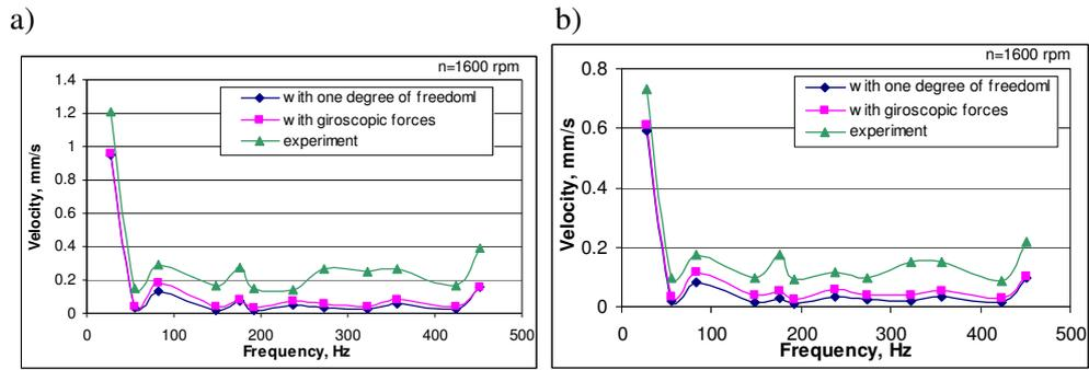
Figure 2.12 Experimental and theoretical results on horizontal (a) and vertical (b) vibrations for blank rotation with gyroscopic forces
