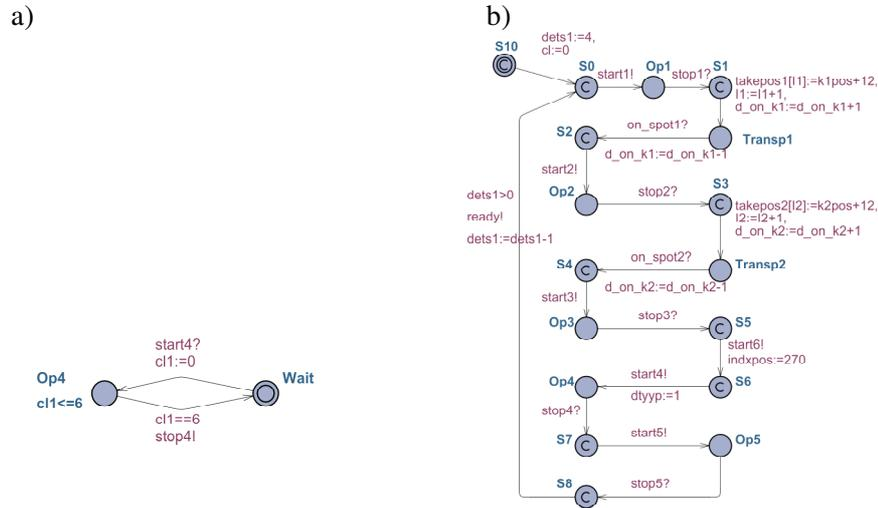
Figure 3.8 Milling machine (a) and detail fragments of FMS as the timed automata models
