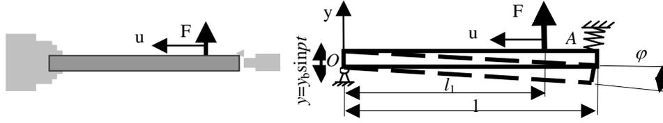
Figure 2.10 Calculation scheme in the case of changing cutting conditions
