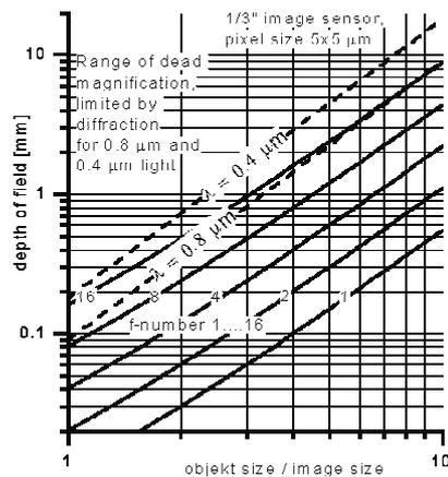
Figure 2.6 Depth of field/magnification curves for the current system
