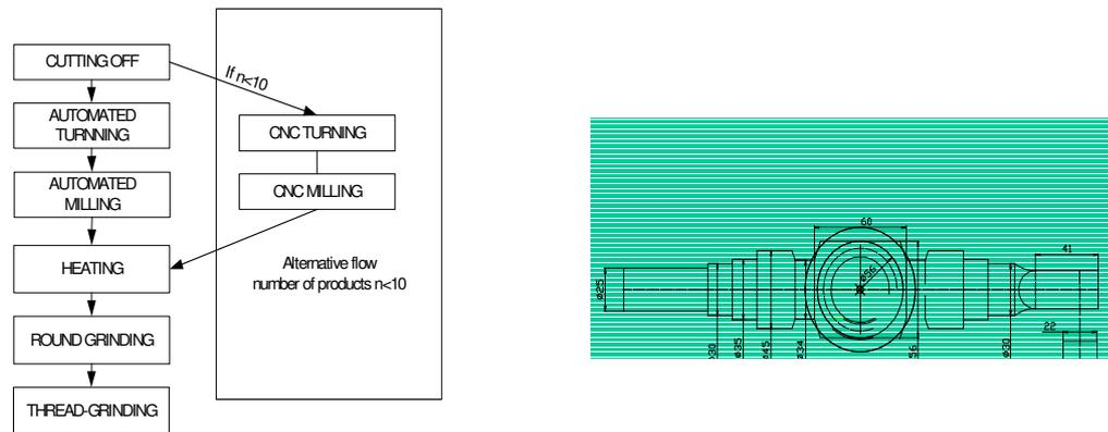
Figure 3.9 An example of trace for manufacturing worm shafts
