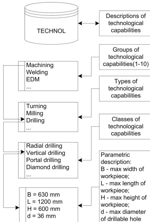
Figure 4.2 Structure of the technological capabilities database Technol
