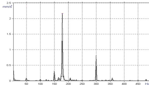
Figure 2.2 Vibrations on CNC lathe
