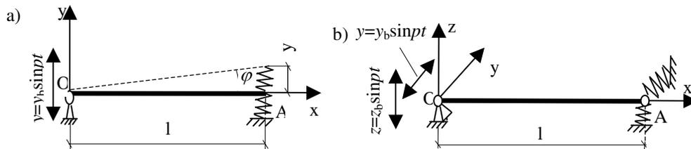
Figure 2.8 Dynamic models with one (a) and two (b) degrees of freedom
