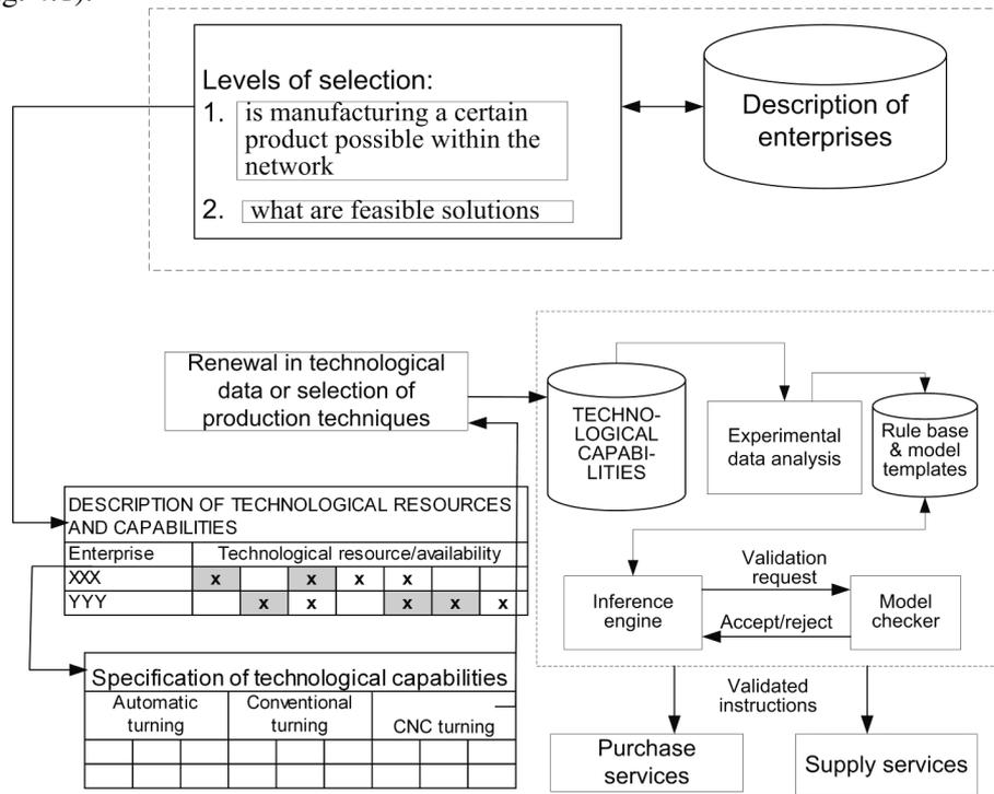
Figure 4.1 Information flow in virtual database solution for planning resource-sharing production in a technological resources network
