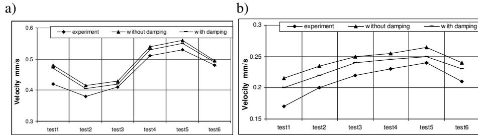
Figure 2.14. Comparative analysis of experimental and theoretical results (dynamical model with two degrees of freedom) for horizontal (a) and vertical (b) vibrations by cutting
