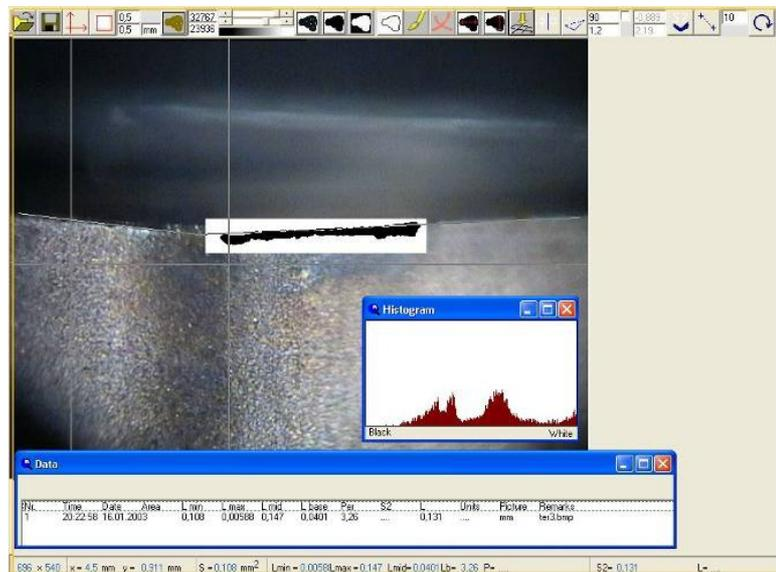
Figure 2.7 Working windows of the image processing program *Terik*
