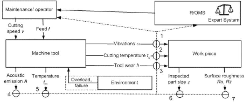
Fig. 3.2 Functional dependencies of IMM modules, where  $\ominus$  – monitored resettable variables of the model
