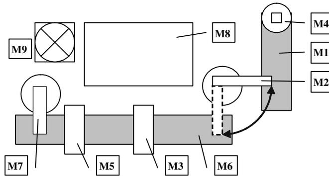
Figure 3.6 Scheme of FMS and modules decomposition
