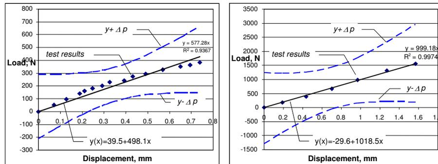
Figure 2.11 Correlation functions between the load and static displacement for horizontal (a) and vertical (b) loads
