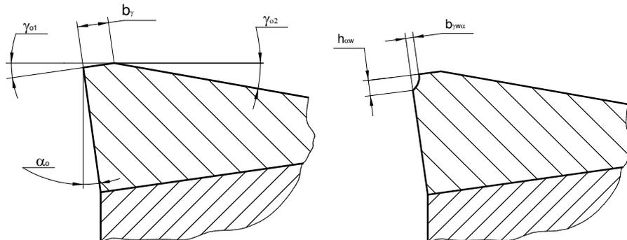
Figure 2.4 An unworn cutter with chamfer honing (a), and a worn cutter at small cutting speeds (b)
