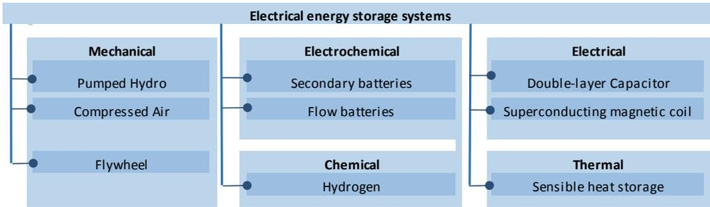
Figure 1.3.1. Classification of electrical energy storage systems according to the energy form
