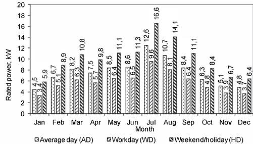
Fig. 4. Rated power of a wind turbine according to the monthly wind speed
