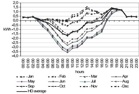
Fig. 5. Balance of HD consumption and generation
