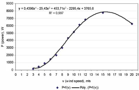
Fig. 3.  $P=f(v)$  characteristic of the chosen wind turbine
