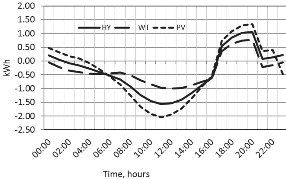
Figure. 3.2.1. Balance of WD consumption and generation
