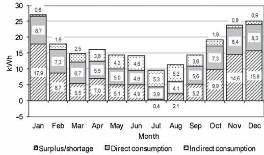
Fig. 8. Direct and indirect load coverage of an average WD of a month
