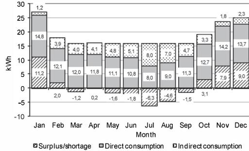
Fig. 9. Direct and indirect load coverage of an average HD of a month
