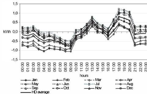
Fig. 6. Balance of HD consumption and generation
