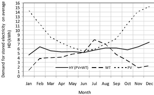
Fig. 9. Average demand for stored electricity for indirect load coverage on an average HD of a month
