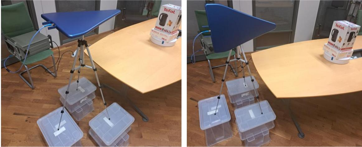
a) Antenna horizontal polarization
