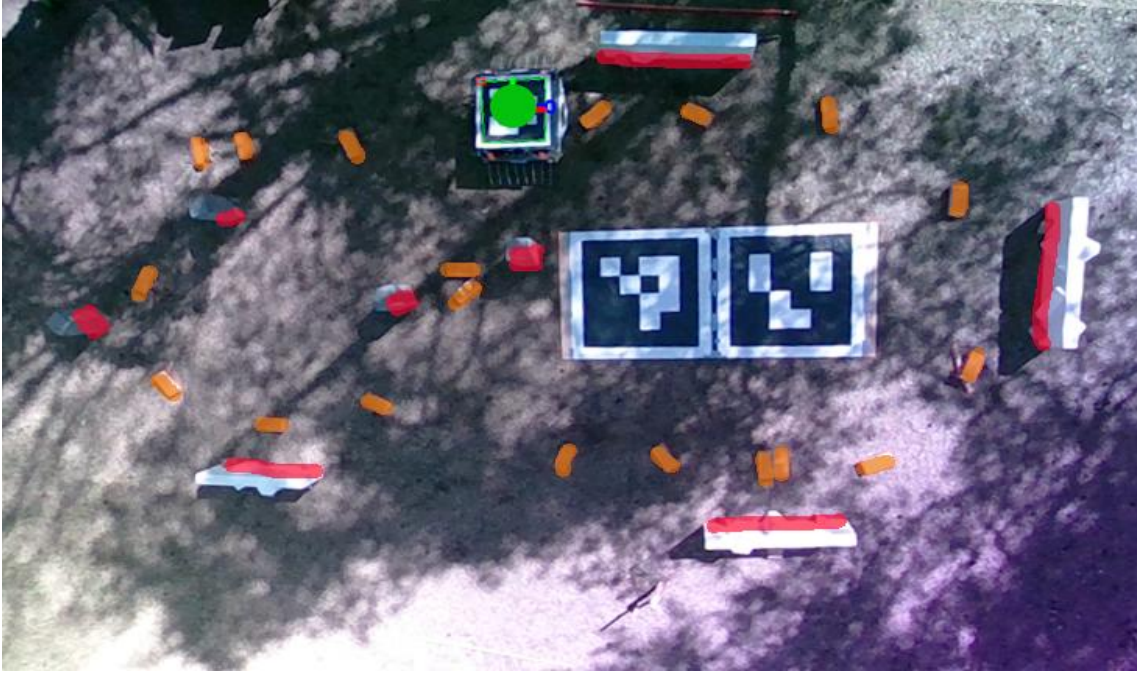
Figure 13. Top view of experiment in real environment. Orange – bricks, red – foam walls and large blocks, green starting position.
