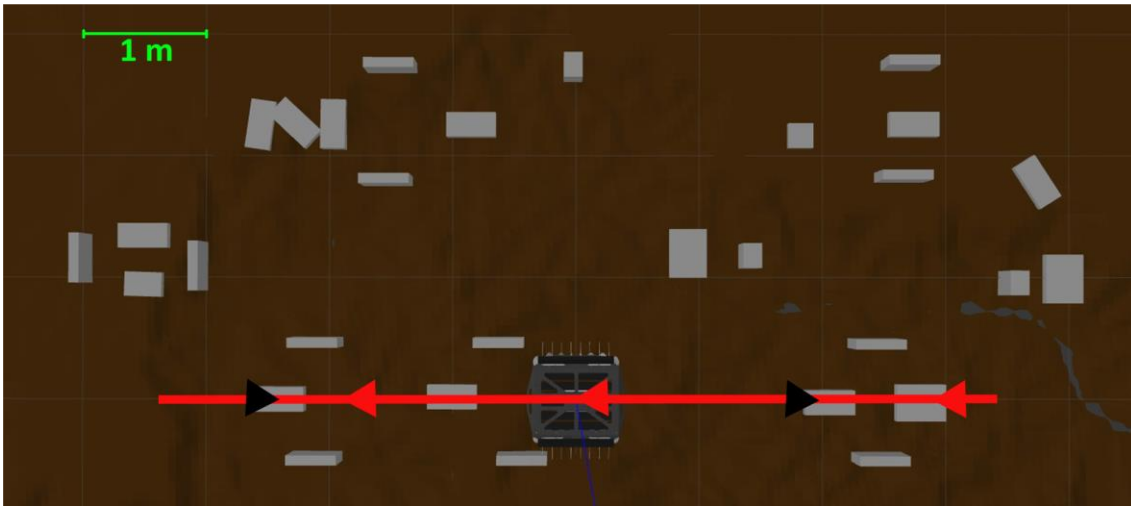
Figure 3. The line track in the simulator. Red arrows show forward moving, black arrows show reversed moving.
