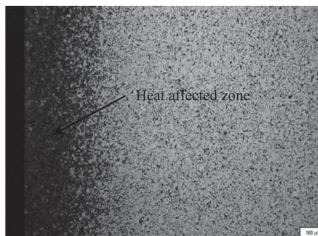
Fig. 1. Heat affected zone of plasma cutting
