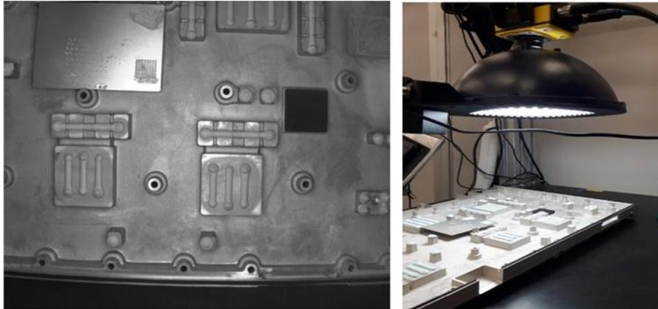
Figure 6.2: Image acquired under diffused dome lighting illumination method
