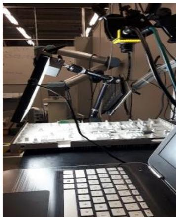
Figure 5.4: Experimental setup for Back Light illumination technique
