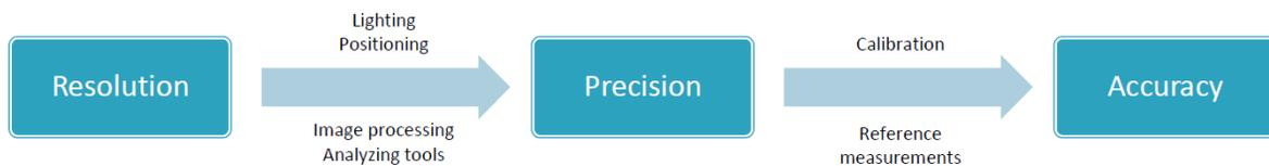
Figure 5.8: Relationship between resolution, precision and accuracy
