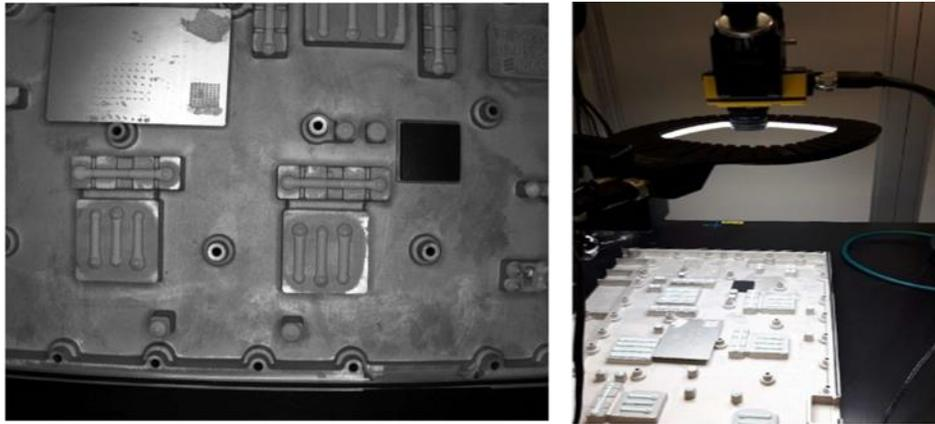
Figure 6.4: Image acquired under Brightfield illumination method
