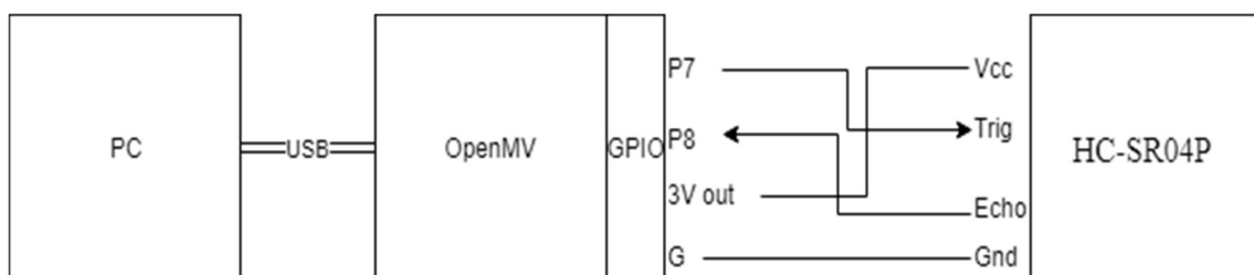
Figure 10. Connection cables between OpenMV and HC-SR04P modules
