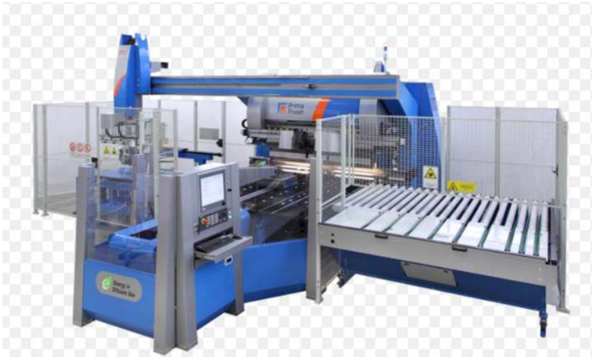
Sele 5.8 Painutusrobot Prima Power Express Bender [16]
