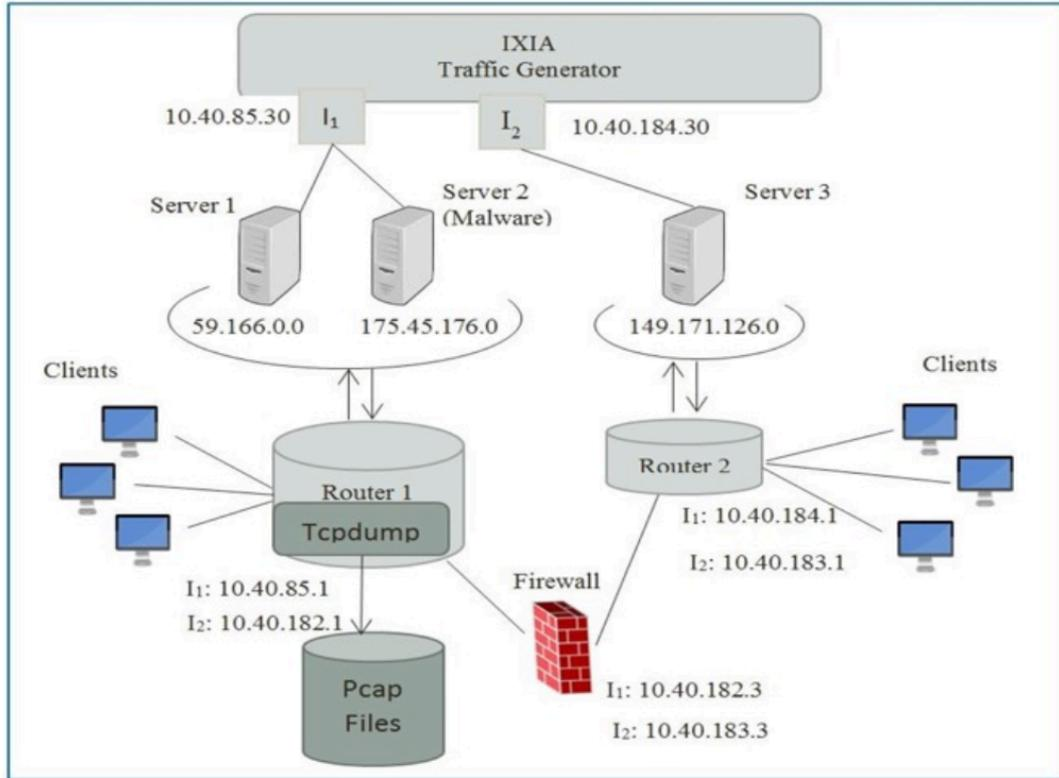
Figure 6. Configuration setup for obtaining the data [5]
