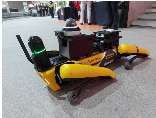
Figure 6. Boston Dynamics SpotMini quadruped robot. Image credit: © David Pérez (DPC), Wikimedia Commons, licensed under CC BY-SA 4.0 [69].
