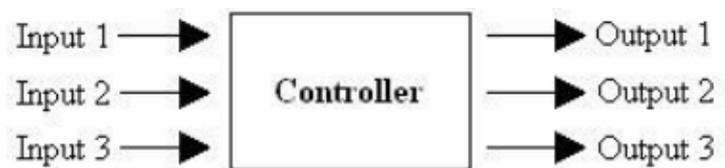
Fig. 2.7. MIMO control scheme
