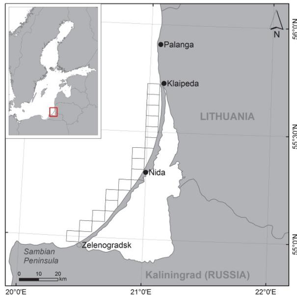
**Figure 10.** Location scheme of the Curonian Spit. Boxes represent the 15 grid cells used in the calculations of sediment flux and the associated coastal sections (Paper V).
