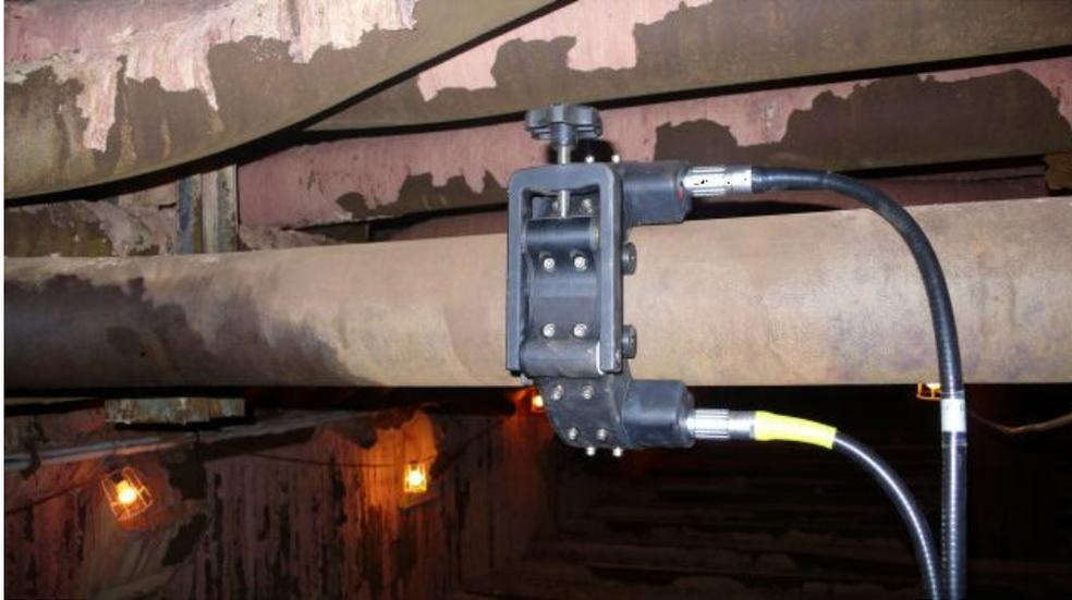
Figure 1. Transducer array employed for guided wave inspection of pipes.
