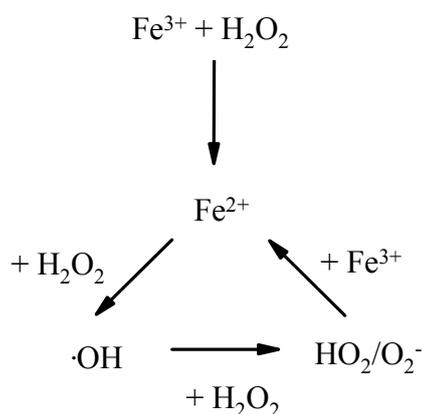
Figure 1.  $\text{Fe}^{3+}$  initiated decomposition of hydrogen peroxide.
