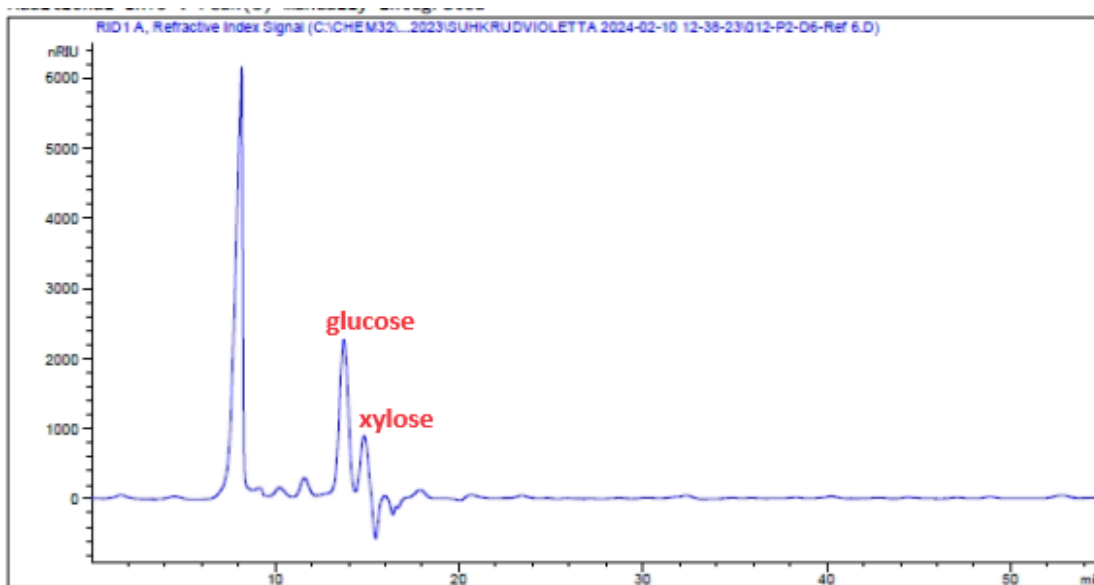
Figure 22. Example chromatogram of cotton analysis via HPLC. Sample: parallel nr 6. Dilution - 0x.
