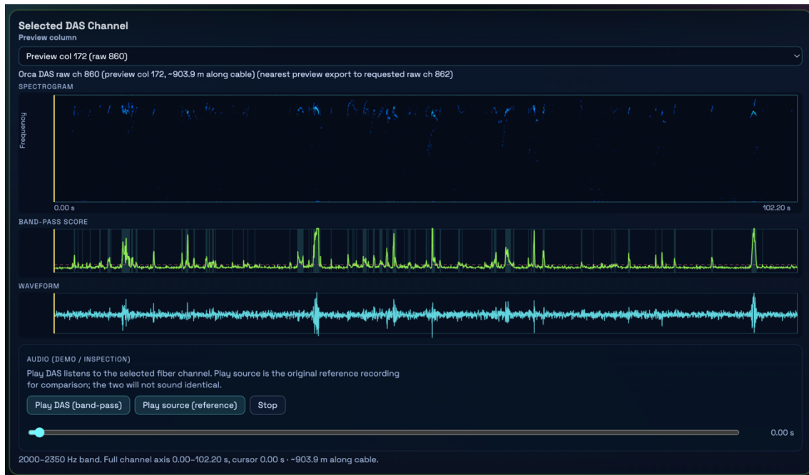
Figure 5-4 Selected-channel inspection panel showing waveform, spectrogram, band-pass score, and source-versus-DAS audio comparison for a selected Orca DAS channel.
