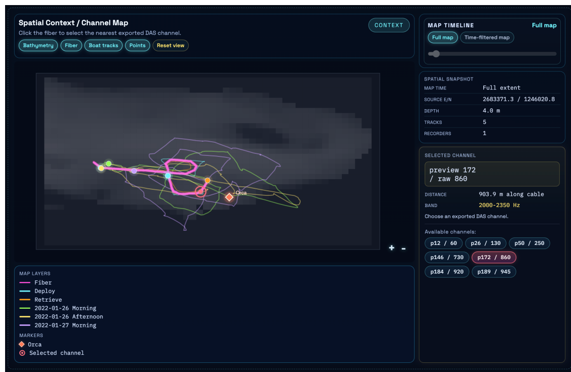
Figure 5-2 Spatial context panel of the interactive viewer showing bathymetry, fiber trajectory, recorder positions, boat tracks, source location, and selected DAS channel.
