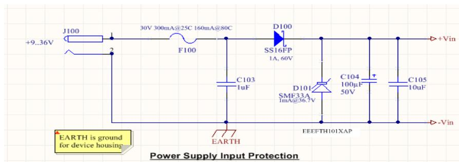
Figure 25: Power supply input for the converters
