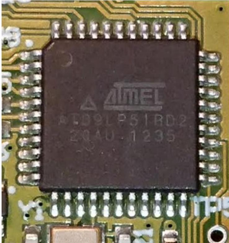
Figure 9: Atmel AT89LP51 microcontroller (8051 architecture), the one that is currently used in ROW
