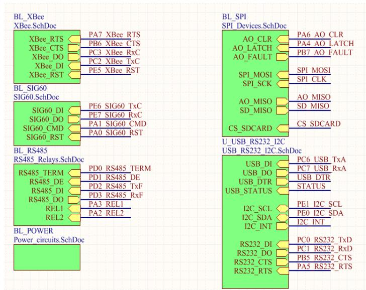
Figure 24: Peripheral blocks
