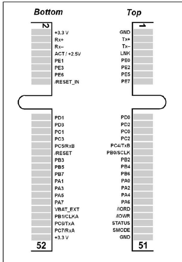
Figure 20: RCM6700 PCI Express header pinout [7]
