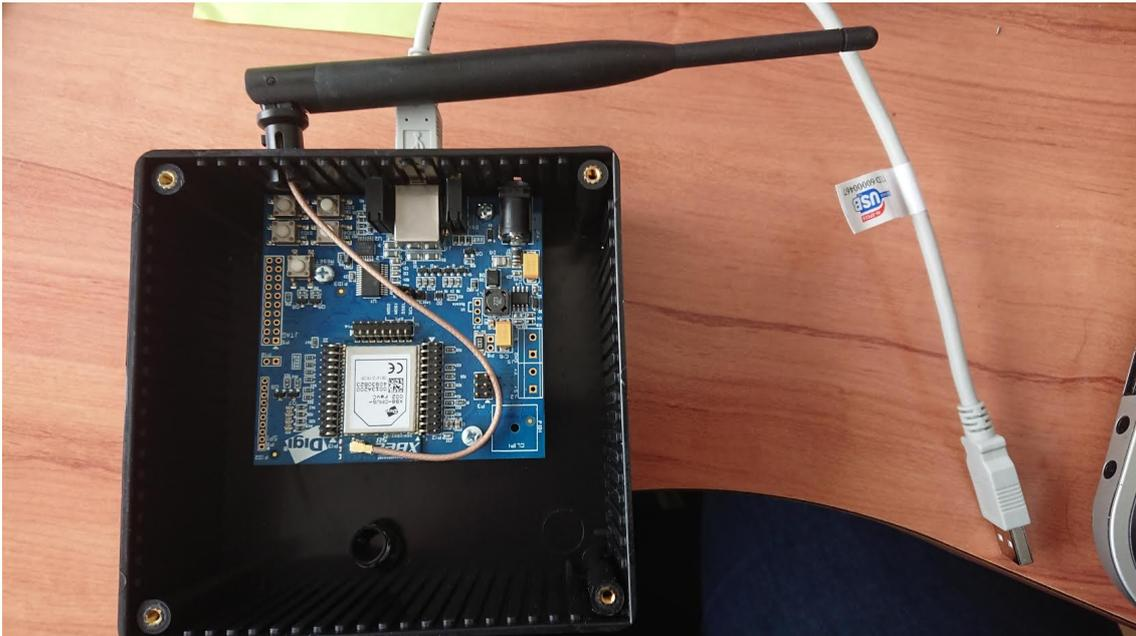
Figure 14: XBee 868LP with a Development kit
