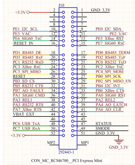
Figure 23: Mini PCI Express header
