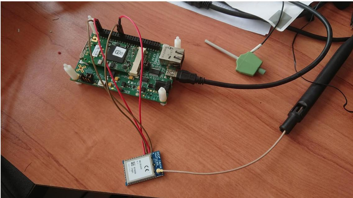
Figure 15: Connecting an XBee SX 868 to an RCM6700 development board for testing
