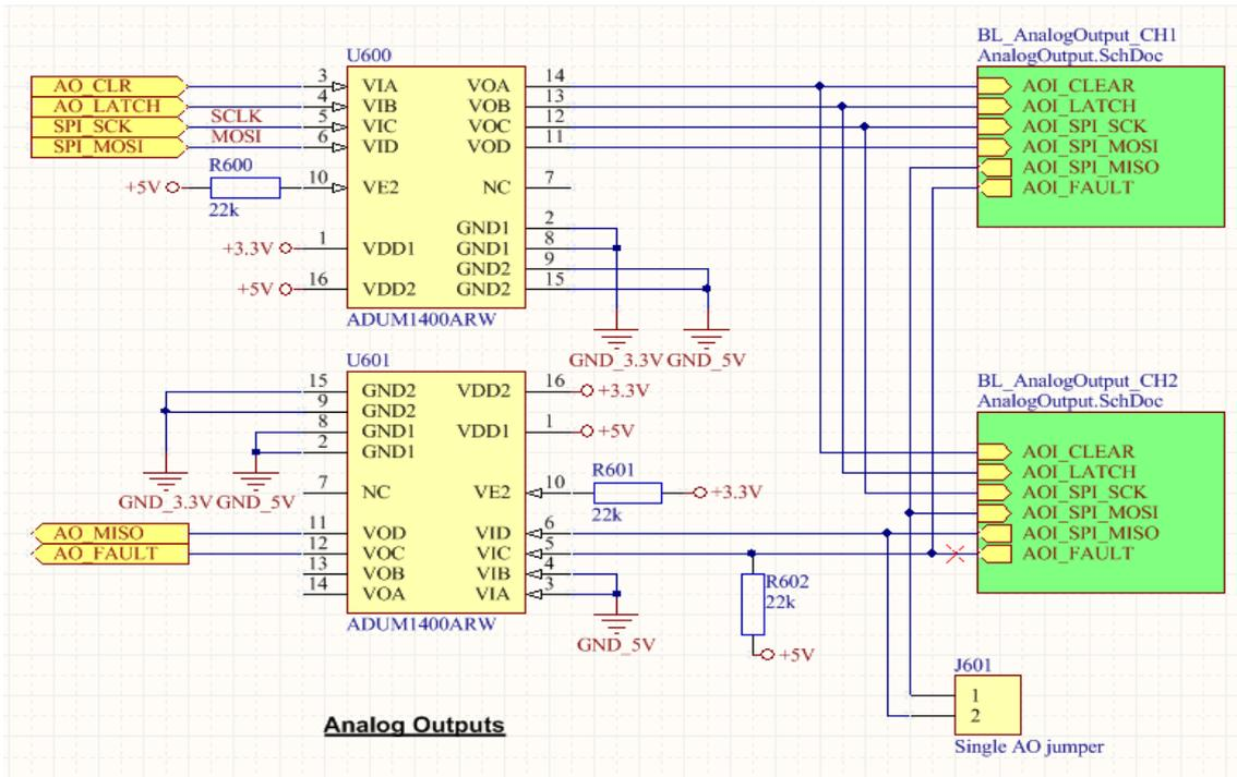
Figure 26: Daisy-chained analog output blocks with galvanic isolation
