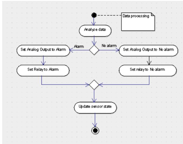
Figure 35: Data processing flowchart
