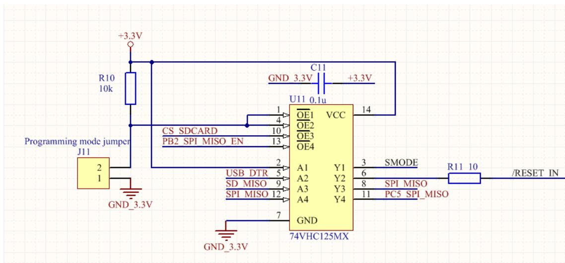
Figure 30: Programming mode jumper and 74VHC125 buffer
