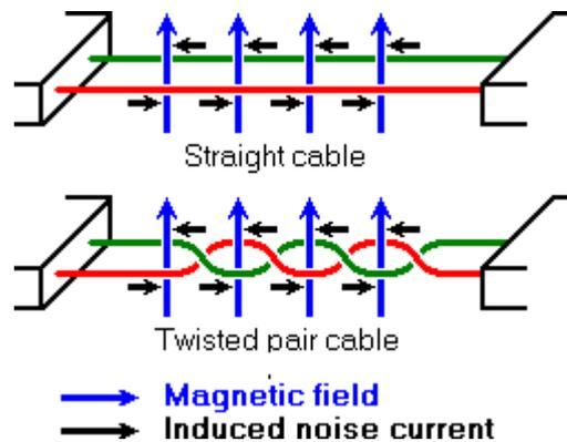
Figure 17: Noise in straight and twisted pair cables [23]
