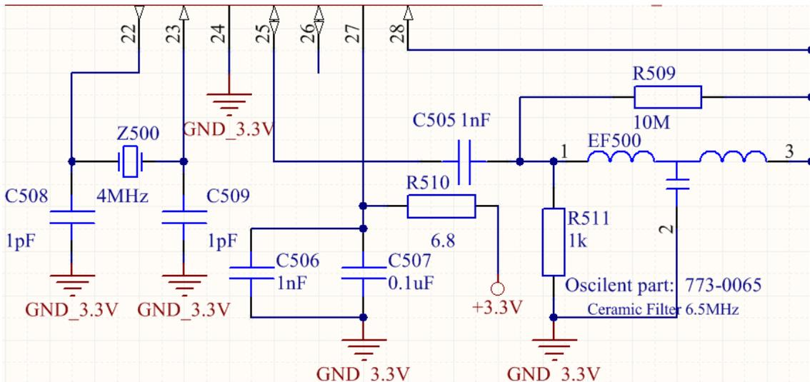
Figure 27: Oscillator, ceramic filter and AVdd connection on SIG60
