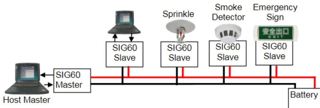
Figure 10: Example of SIG60 in fire protection network [15]
