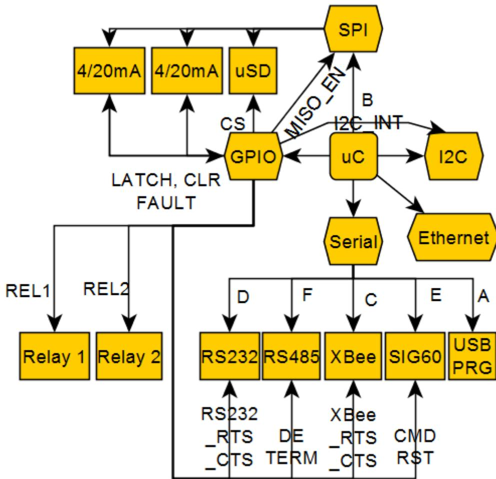
Figure 19: Block scheme of interfaces and pin requirements
