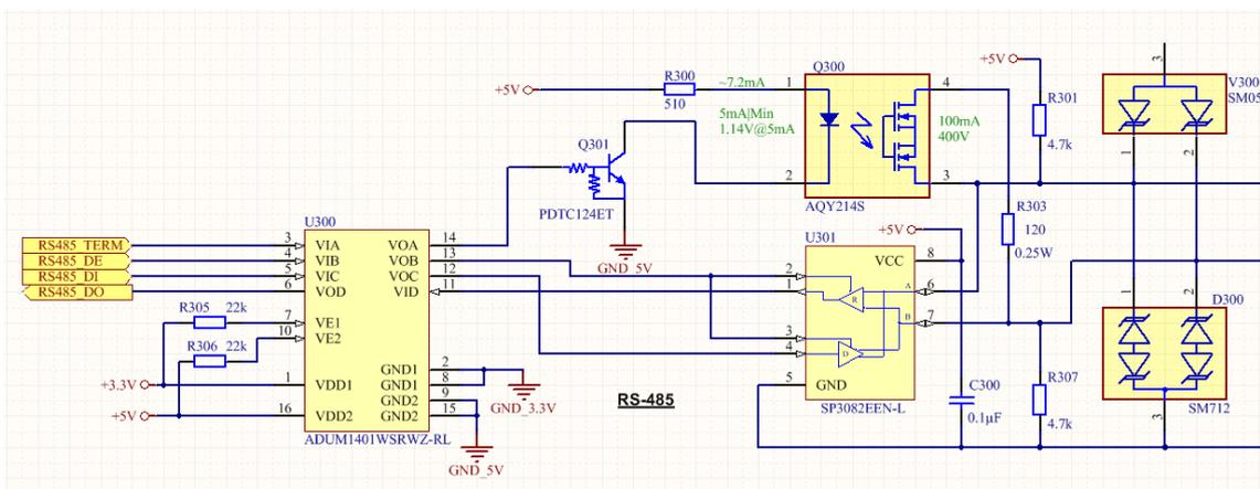
Figure 28: RS-485 circuitry with terminal resistor relay and galvanic isolation
