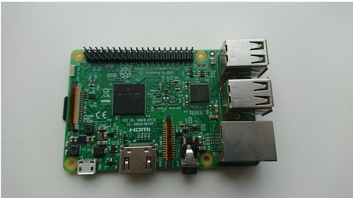
Figure 6: Raspberry Pi 3 Model B
