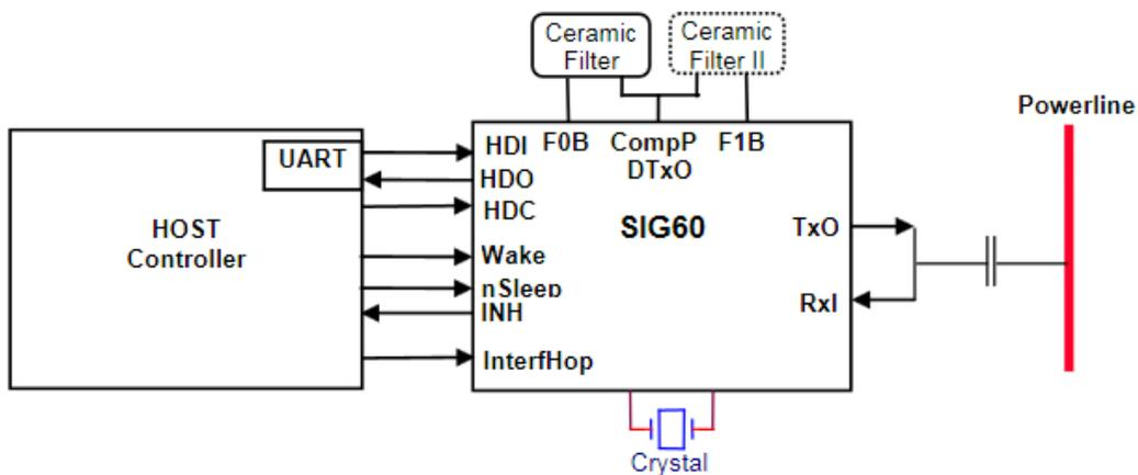
Figure 12: SIG60 interfacing and external components [15]
