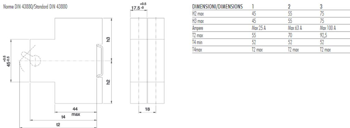
Figure 21: Enclosure dimensions according to DIN 43880 [28]
