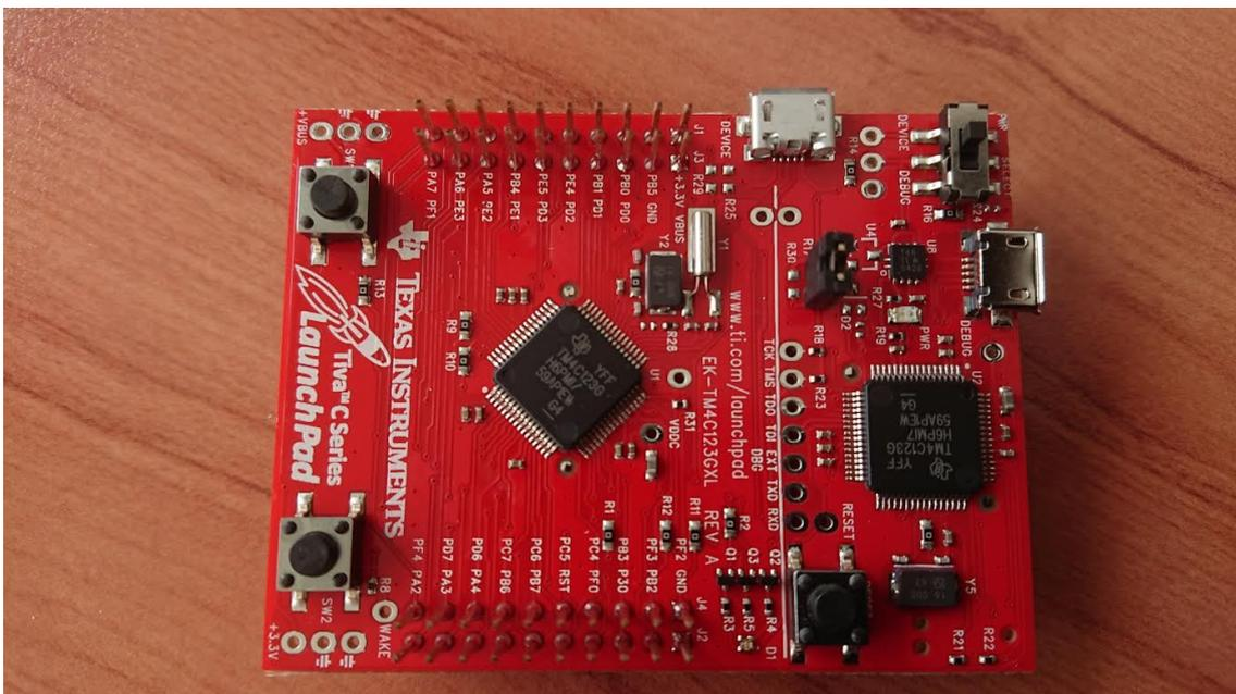
Figure 8: Texas Instruments LaunchPad with a TMC123G controller based on ARM Cortex-M4 series. This LaunchPad contains an additional microcontroller for programming and debugging.
