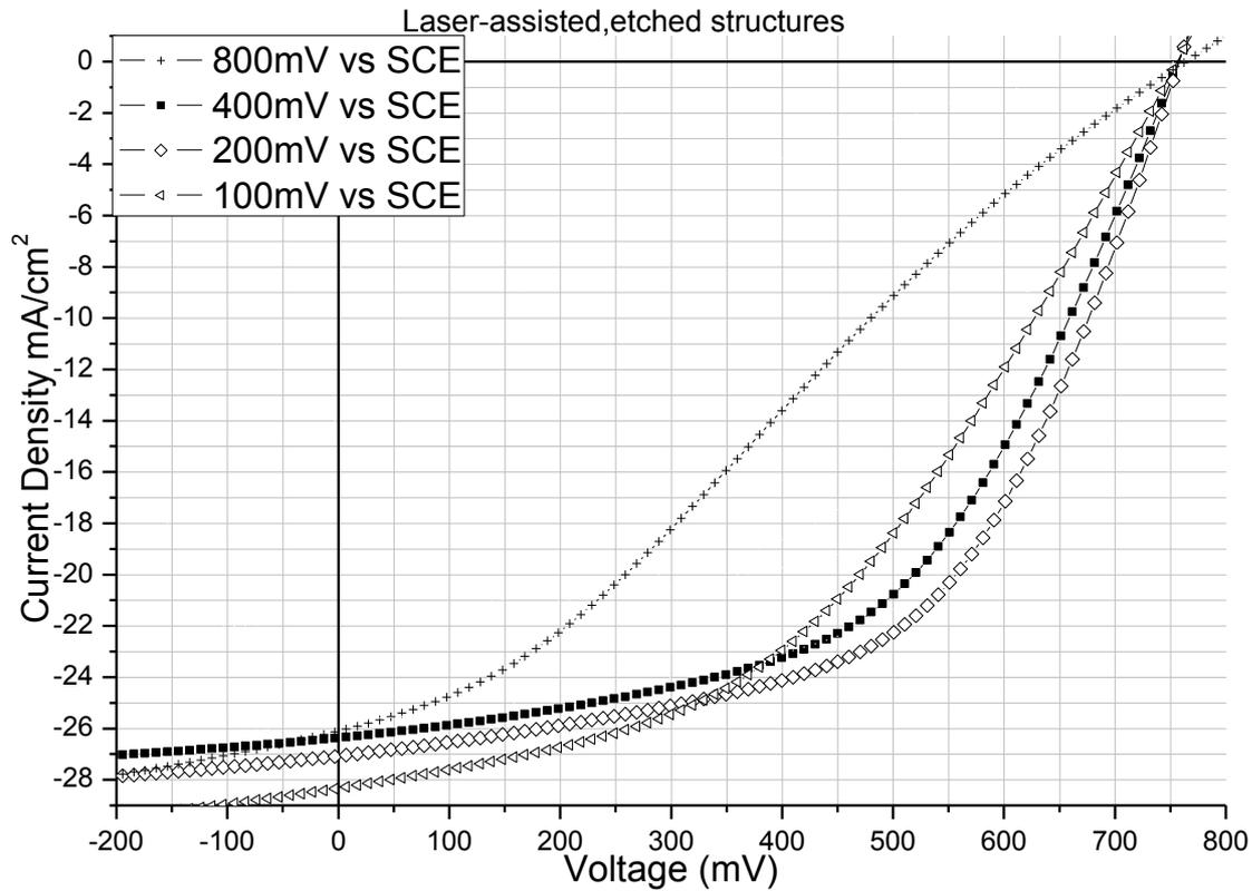
**Figure 16.** I-V curves of PPy:PTSA/CdTe/CdS/SnO<sub>2</sub>/ITO/glass hybrid structures coated with electrodeposited PPy: PTSA layers under laser illumination at the applied potential range from 100 to 800 mV vs. SCE.
