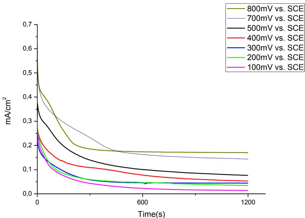
**Figure 10.** Electrodeposition curves of PPy: PTSA layers onto CdTe layer in ACN solution under laser beam illumination with an intensity of 20 mW/cm<sup>2</sup>.
