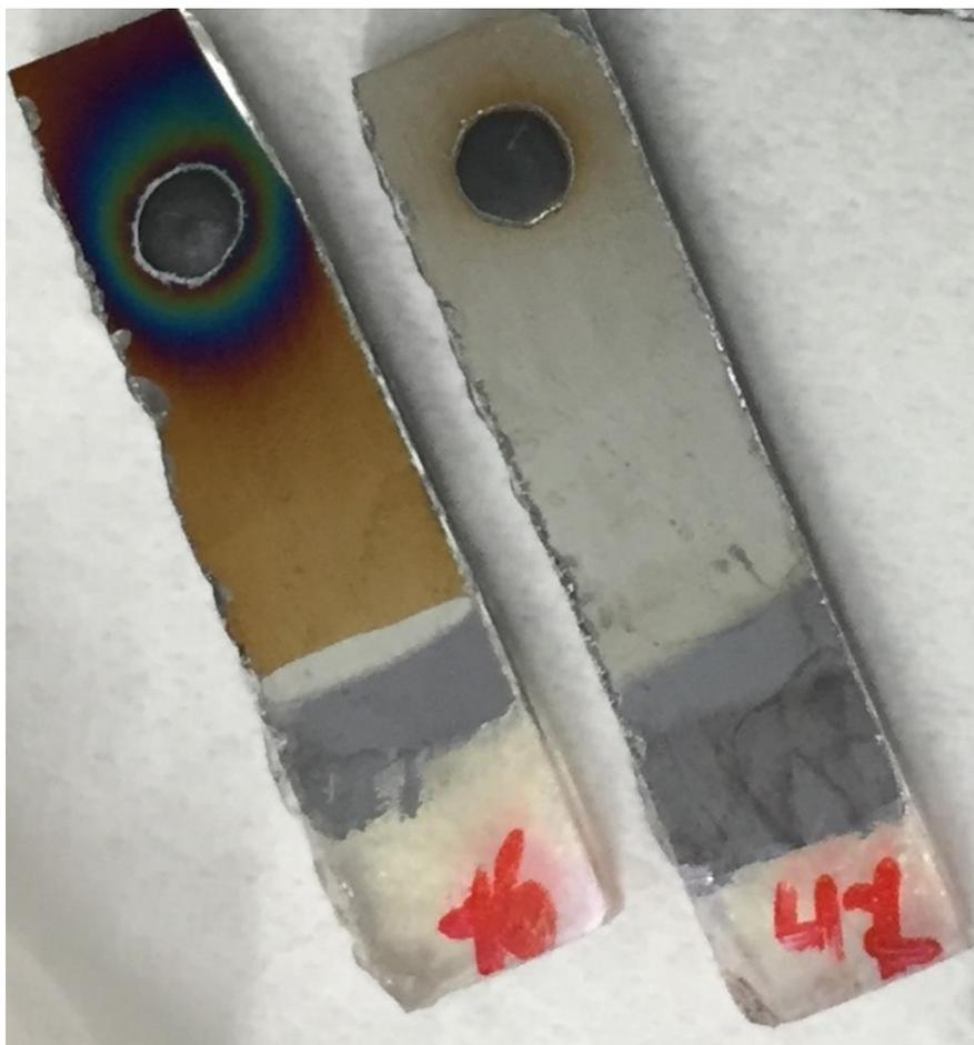
**Figure 11. Photograph of scribed samples of** graphite/PPy:PTSA/CdTe/CdS/SnO<sub>2</sub>/ITO/glass structures (from left to right – PPy deposited at 700mV and 200 vs. SCE).
