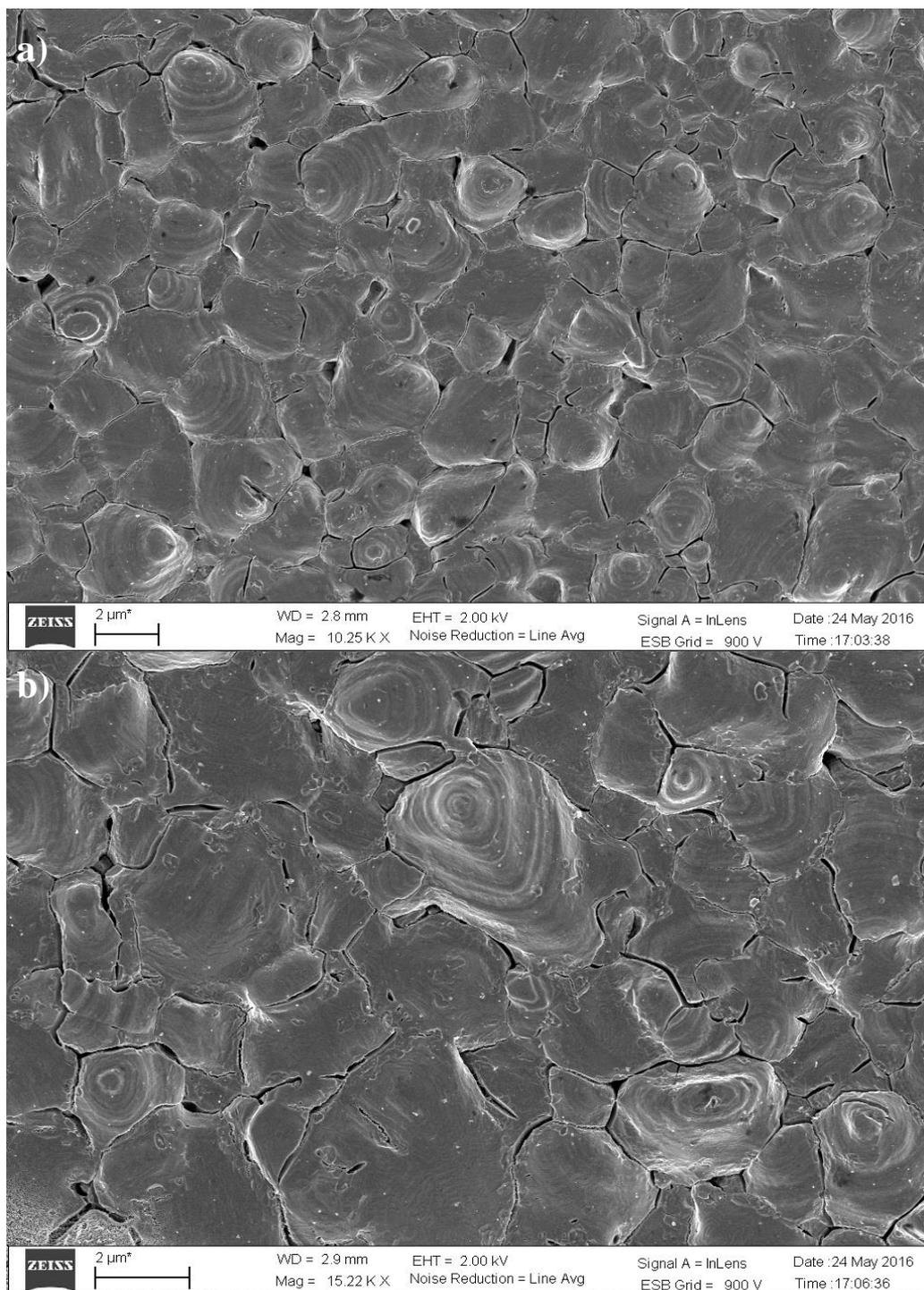
**Figure 12 (a, b).** HR-SEM image of CdTe surface of CdTe/CdS/SnO<sub>2</sub>/ITO/glass structure etched in NP-acid during 30 sec.
