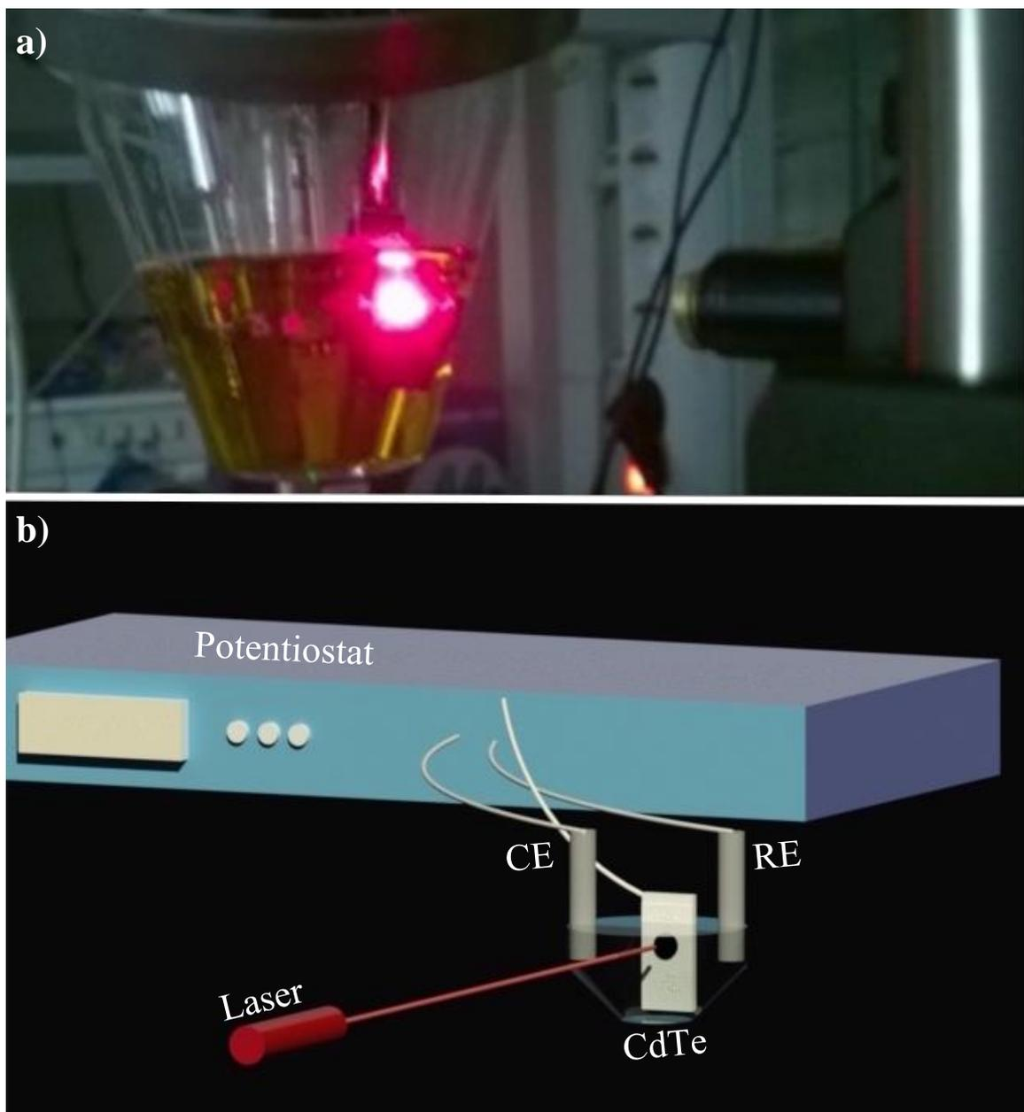
**Figure 9** (a) – Photograph of electrochemical cell irradiated with laser and (b) – schematic drawing of setup for photoassisted electrodeposition.
