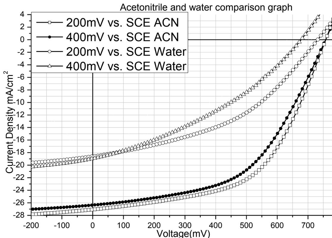
**Figure 18.** I-V curves for complete hybrid structures PPy/CdTe/CdS/SnO<sub>2</sub>/ITO/glass with electrodeposited PPy: PTSA back contact layer in ACN media and PPy:  $\beta$ -NSA back contact layer electrodeposited in aqueous media under laser illumination at the potentials 200 and 400 mV vs. SCE (all I-V curves were measured under white light irradiation of 100 mW/cm<sup>2</sup> intensity).
