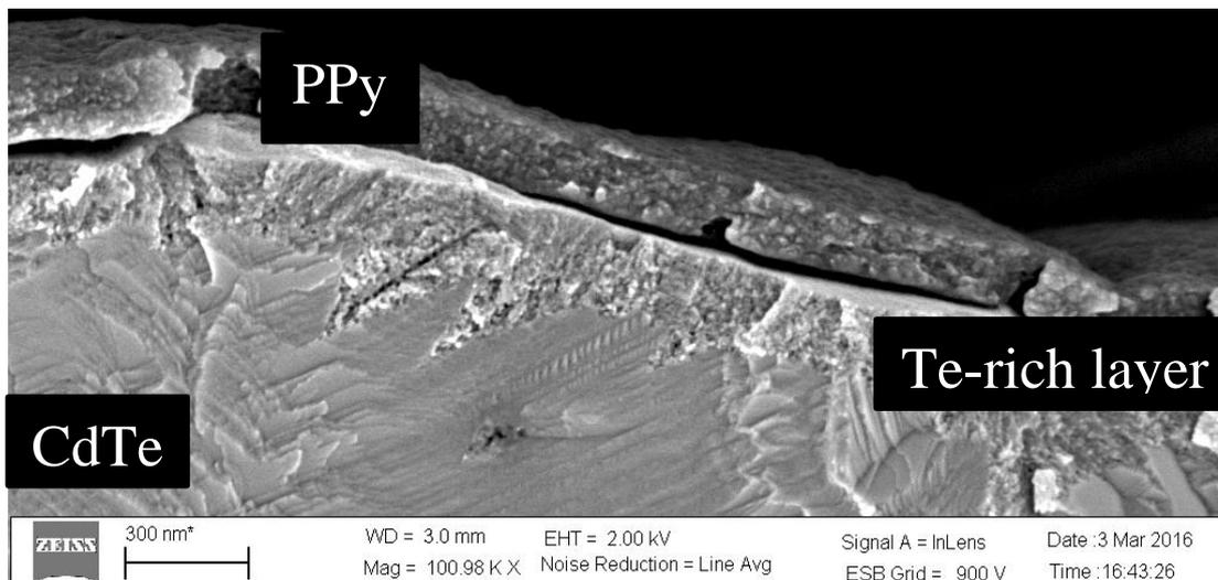
**Figure 14 (a, b, c, d).** Cross sectional HR-SEM micrograph at different magnifications of PPy:PTSA/CdTe/CdS/SnO<sub>2</sub>/ITO/glass structure with PPy film deposited at 400 mV vs. SCE for 20 min at room temperature under laser illumination in ACN solution.
