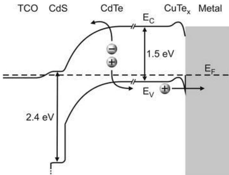
**Figure 2.** Energy band diagram of TCO/CdS/CdTe/CuTe<sub>x</sub>/Metal solar cell [27].
