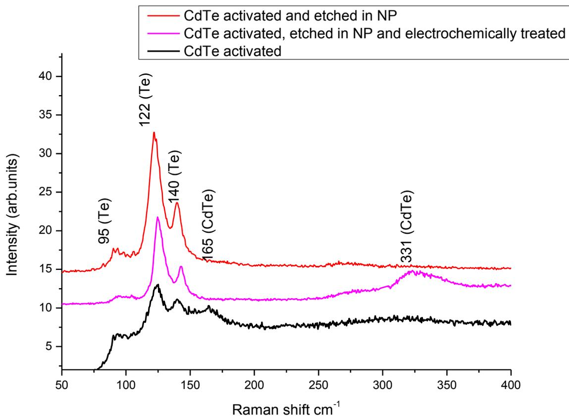
**Figure 15.** Raman spectra of activated CdTe surface; CdTe activated and etched in NP; CdTe activated, etched in NP and electrochemically treated in 0.1M PTSA solution in ACN during 20 min at applied potential of 200 mV vs. SCE.
