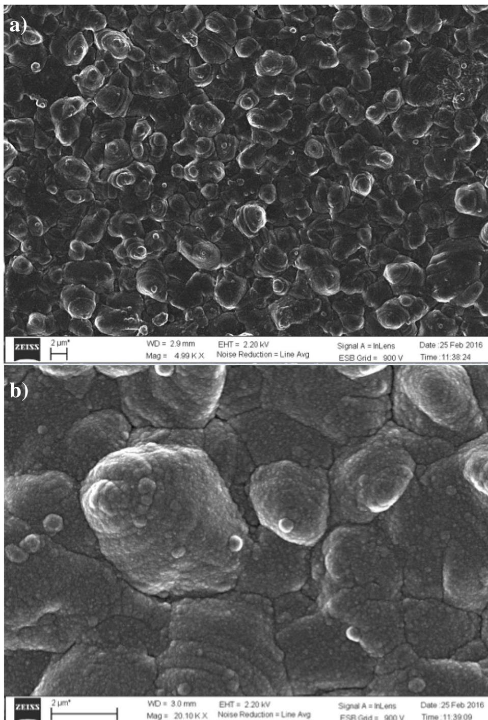
**Figure 13 (a, b).** HR-SEM surface image of PPy:PTSA layer in PPy: PTSA/ CdTe/CdS/SnO<sub>2</sub>/ITO/glass structure (PPy film deposited at 200 mV vs. SCE for 20 min in ACN solution at room temperature under laser illumination).
