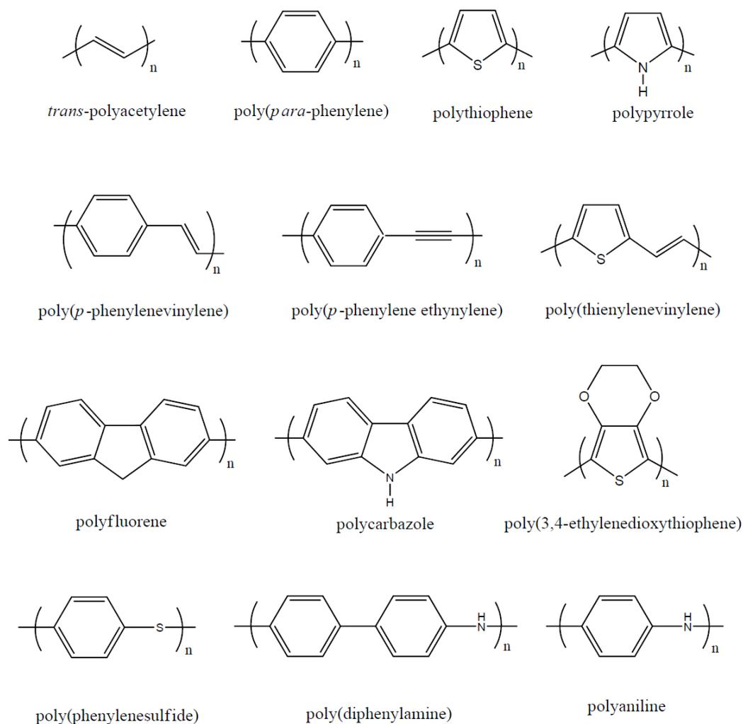
**Figure 5.** Main monomer structures of ECPs [37].
