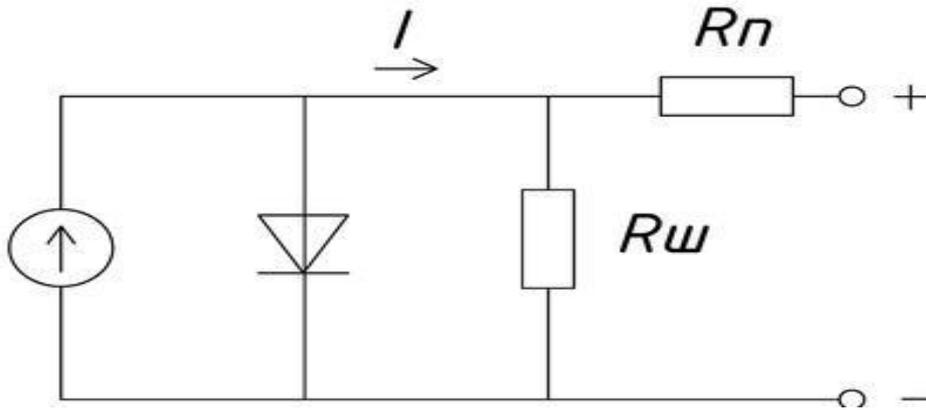
**Figure 3.**The equivalent circuit of the solar cell [28].
