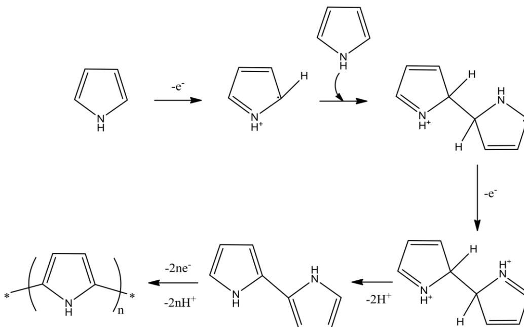
**Figure 6.** Mechanism of chemical synthesis of PPy [42].
