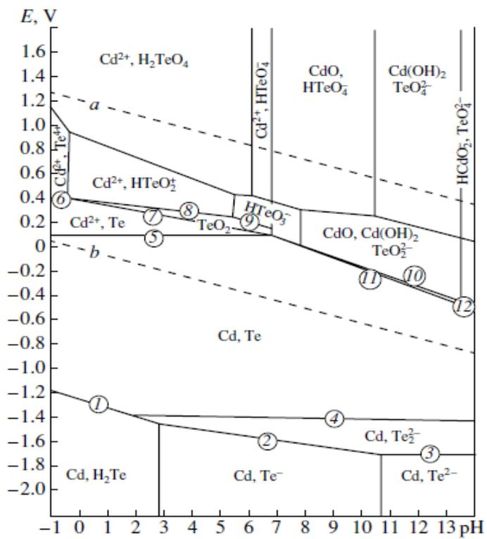
**Figure 17.** Pourbaix diagram of CdTe-H<sub>2</sub>O system (potential is given vs. NHE).
