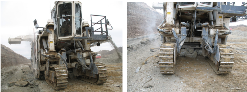
Figure 11. Effect of cutted rock oversizing. when h/V ratio > 6\%
