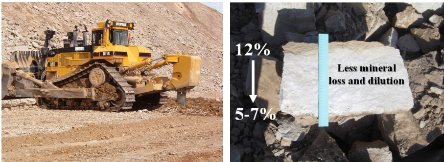
Figure 13. The Ripper-dozer at ripping and oil-shale losses on contact with limestone layer (C/D).
