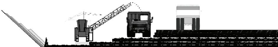
Figure 2. Different loading technologies: windrowing (A.) and direct truck loading with Wirtgen 2500SM (B.)
