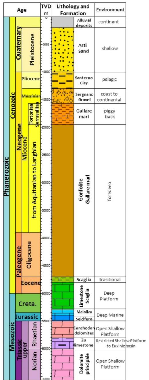
Figure 4. Lithological section of the Sergnano gravel reservoir with sonic log, spontaneous potential and porosity from Malossa B well. Stratigraphic chart on the right side (Colucci et al., 2016).
