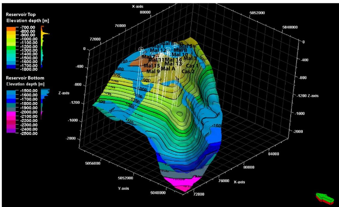
Figure 6. 3D model of the top and bottom of the Sergnano gravel reservoir. The high transparency of the top reservoir allowed to examine where the bottom reservoir merges with the top.
