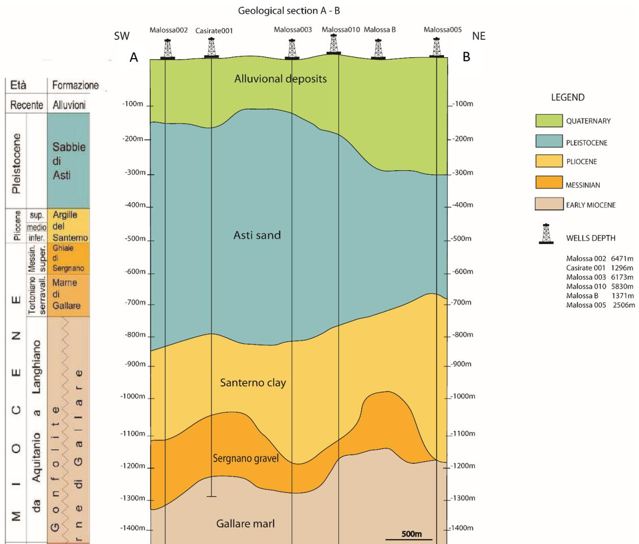
Figure 11. Geological cross section along the A–B line shown at the Figure 6. Stratigraphic chart from Guandalini et al. (2010).
