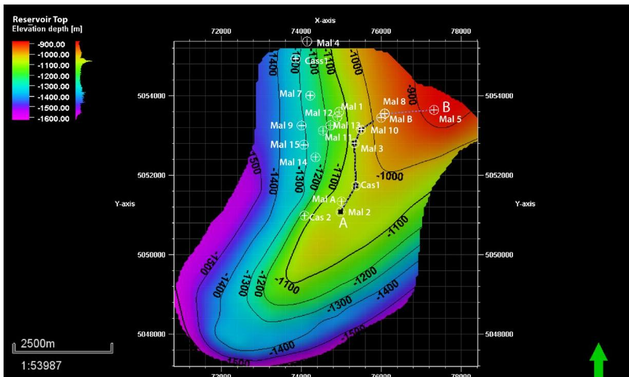
Figure 8. 2D contour map of the Sergnano gravel reservoir top with wells and cross section line A–B.
