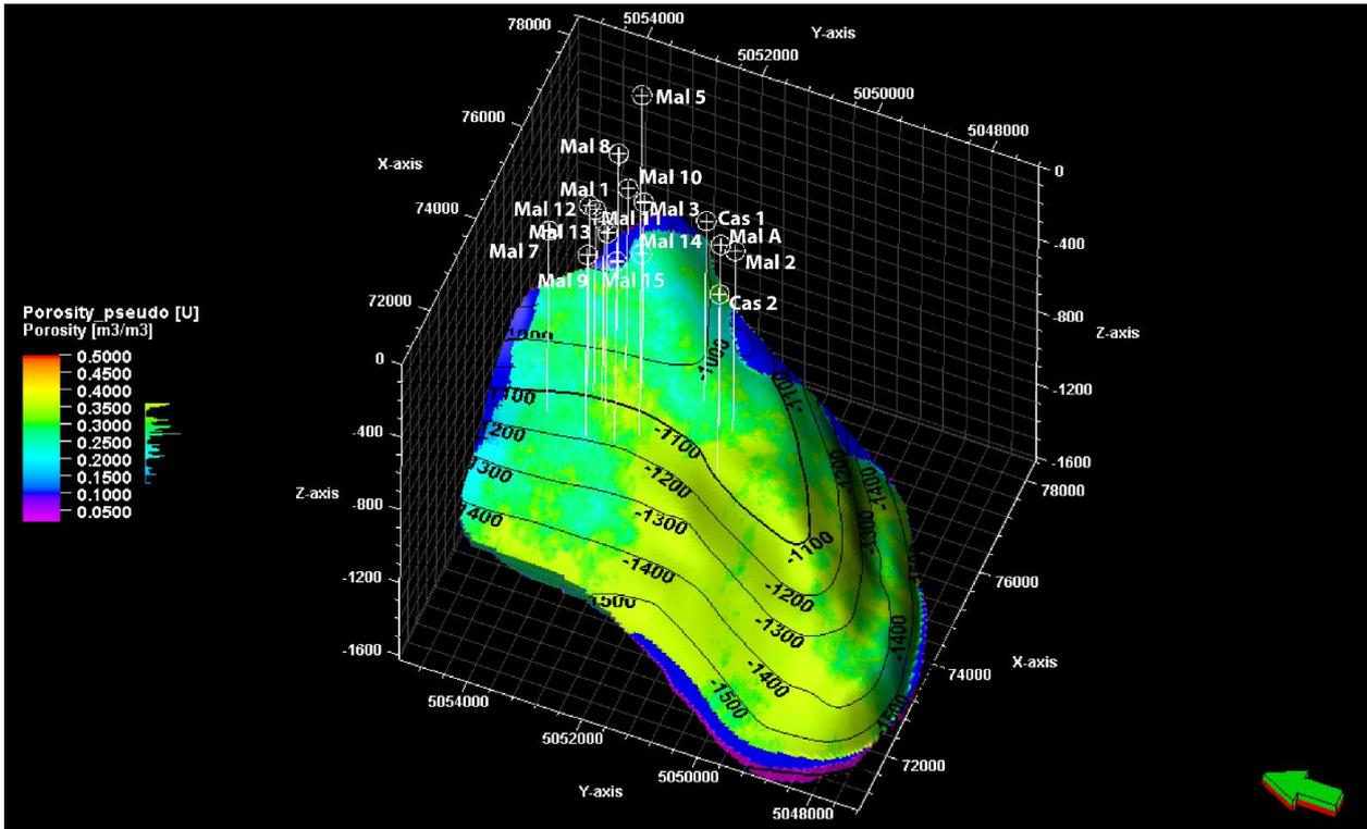
Figure 9. 3D model of the Sergnano gravel reservoir Formation top filled with the porosity data.
