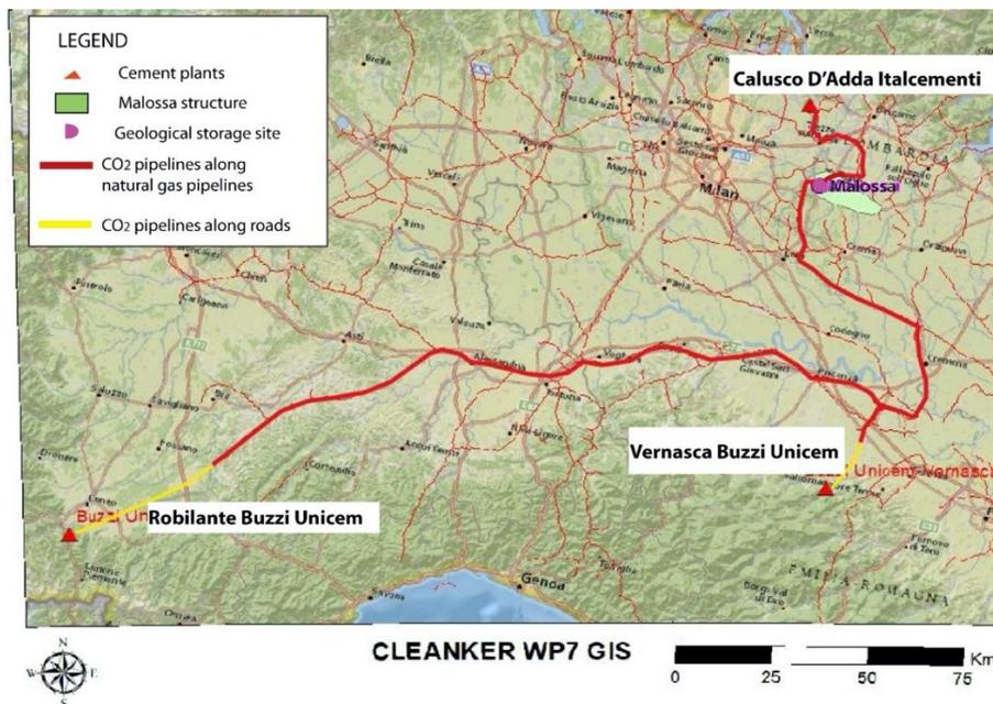
Figure 13. Proposed CO<sub>2</sub> pipelines constructed along available roads and natural gas pipelines.
