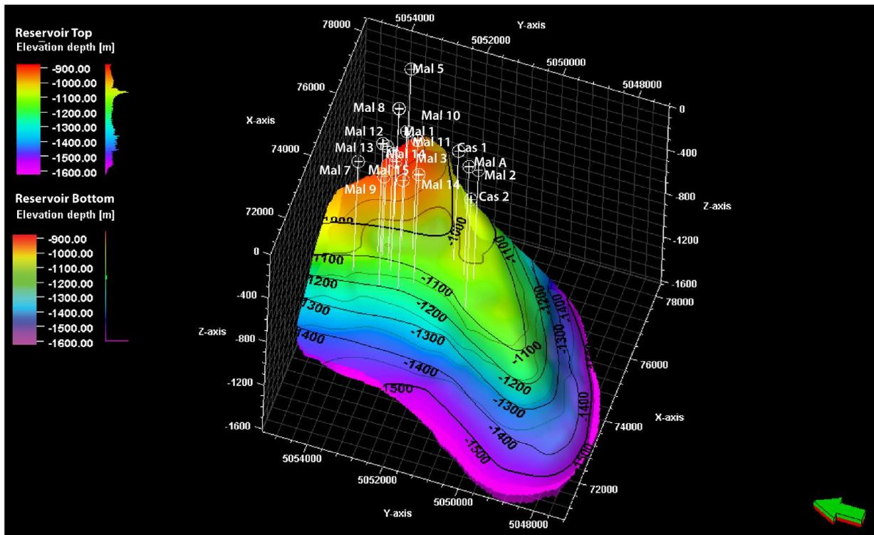
Figure 7. The final version of the 3D geological model of the Sergnano Gravel reservoir Formation top and bottom.
