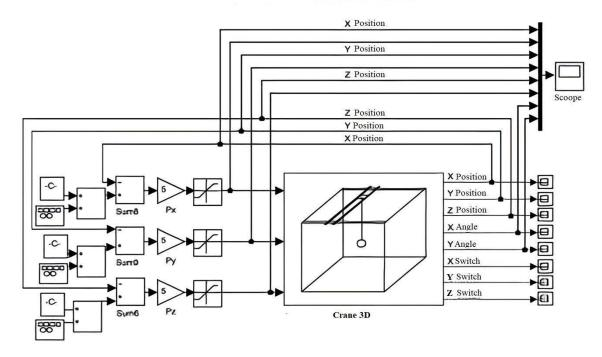
Figure 3. A Simulink model implementing a P controller to control the position of the payload in threedimensional space for the 3D Crane control object investigated in this thesis.
