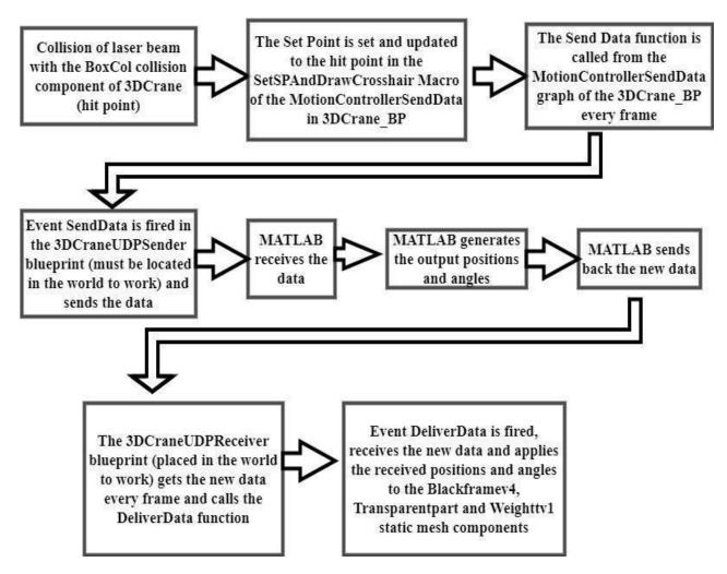
Figure 4. Implementation in UE4 for the 3DCrane\_BP.
