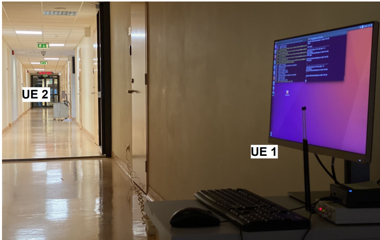
Figure 16: UEs perform ProSe direct discovery in an indoor LoS transmission path (corridor).
