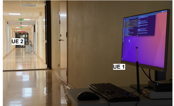
FIGURE 9. UEs perform ProSe direct discovery in an indoor LoS transmission path (corridor).
