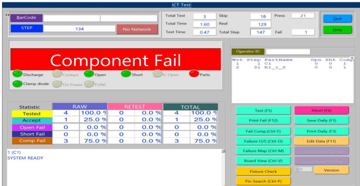
Figure 2.8 Mass production FAIL view.
