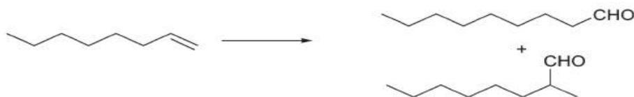
Figure XV: products of the hydroformylation of 1-octene
