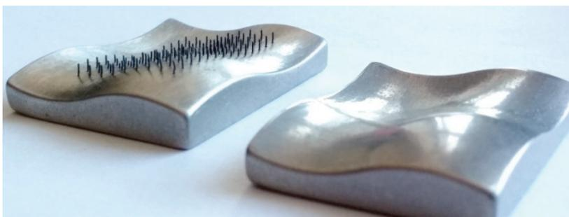
Figure 4.7 Pin structure deposited via DED on the curved surface.
