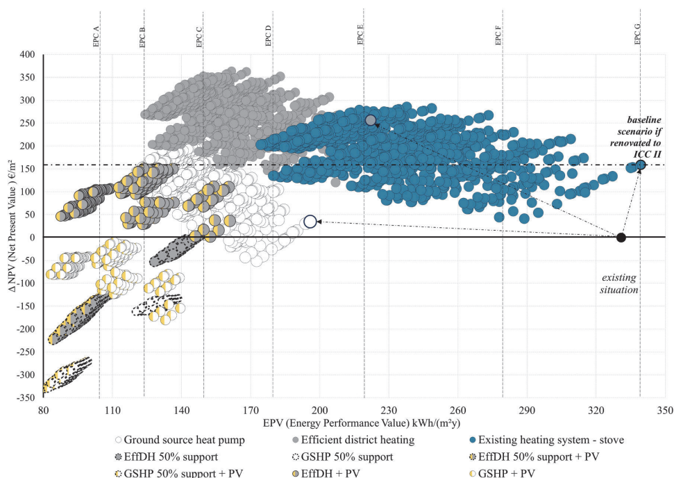
Fig. 6. The dependence of net present value on the energy performance of the building with three heat sources for heating rooms, ventilation aid, and DHW. The black marker refers to the current situation. Scenarios are looked at as if the base case is a stove heating system and compared with a change to GSHP and EffDH solutions. The lowest value with EffDH and GSHP is gained with a 50% grant to support the renovation. The size of the bubble refers to a renovation solution's embodied carbon footprint value, yellow colour indicates PV panels affect in the solution.
