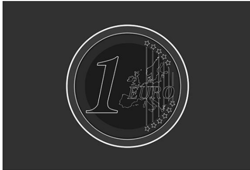
Figure 2.3 How edges emphasize through darkfield [11]
