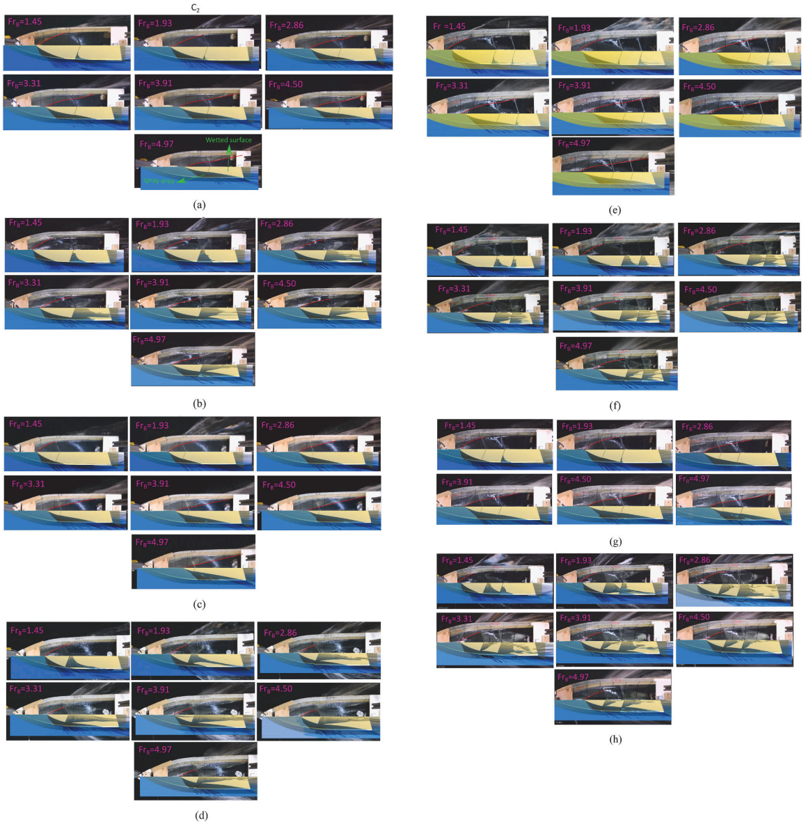
Fig. 8. Comparison of the numerically calculated wetted surfaces against the experimental results of Vitiello et al. (2022): a) C02, b) C03, c) C04, d) C05, e) C06, f) C07, g) C08, and h) C09.
