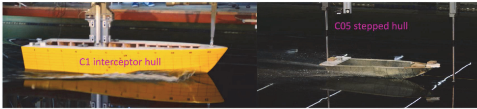
Fig. 1. Set-up of resistance towing tank tests for the C1 interceptor hull (left) and the C05 stepped hull (right) at the Università degli Studi di Napoli "Federico II" Towing Tank (De Luca and Pensa, 2017; Vitiello et al., 2022).
