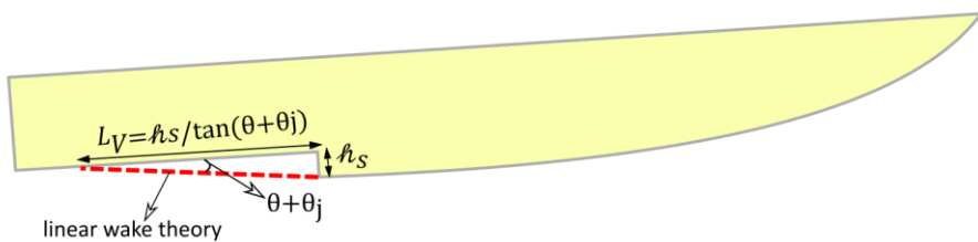
Figure 8. The schematic of linear wake profile assumption.
