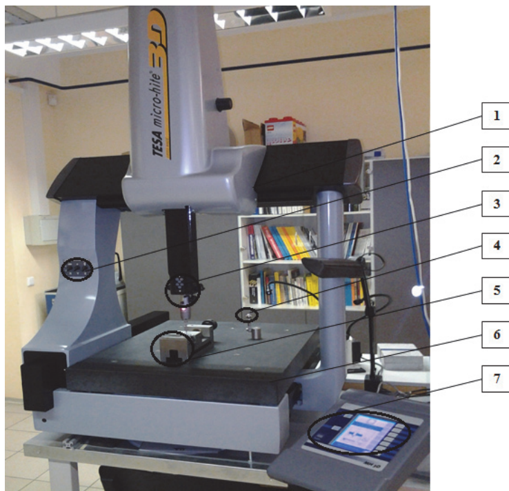
Figure 2.3 Layout of the measurement setup: 1 – moving bridge; 2 – guide in 3D (X/Y/Z); 3 – exchangeable probe accompanied with probe command button; 4 – calibration ball; 5 – workpiece place; 6 – measuring range volume; 7 – software controller
