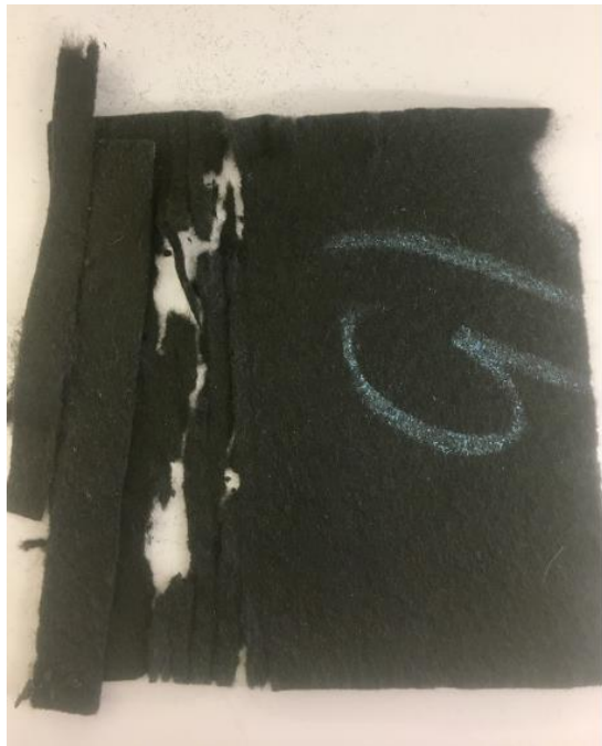
FIGURE 3.9 SAMPLE S5 DEGRADATION RECORDED DURING THE TEST ANALYZATION
