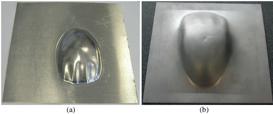
Fig. 4.14. Mouse part: (a) produced by positive forming; (b) produced by negative forming
