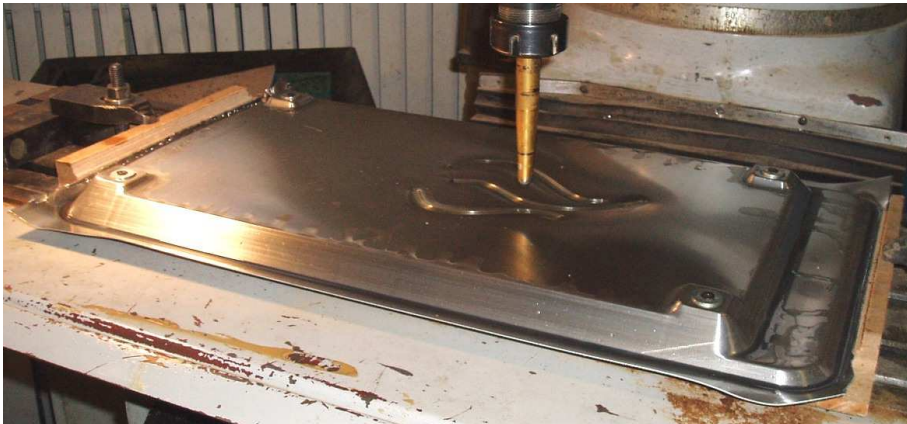
Fig. 4.10. Forming of the cooker casing in CNC milling machine
