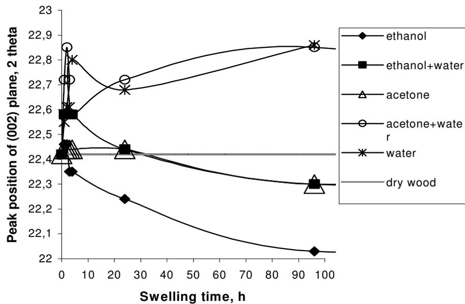
**Figure 5.25.** Shift of the peak position in the (002) plane during swelling of wood in various solutions
