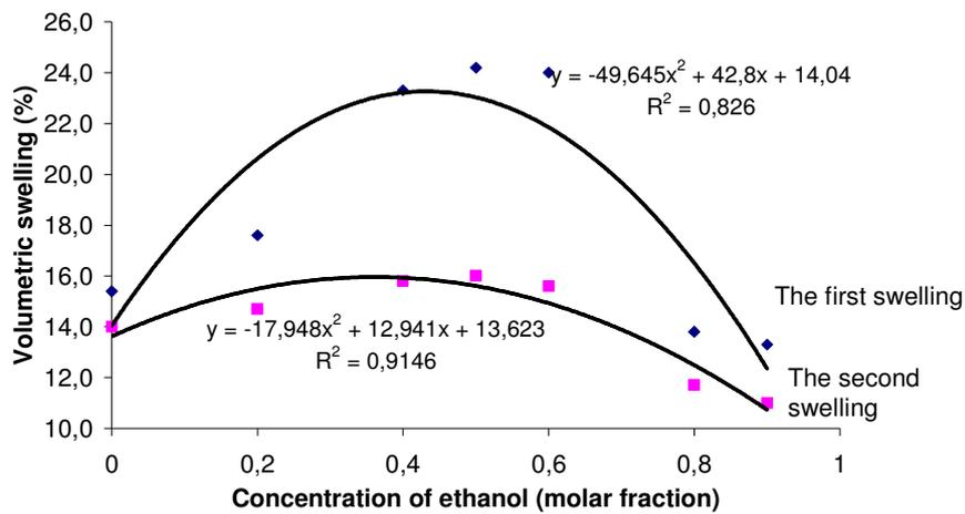
**Figure 5.10.** Repeated swelling of pine sapwood in aqueous solutions of ethanol (new solutions)
