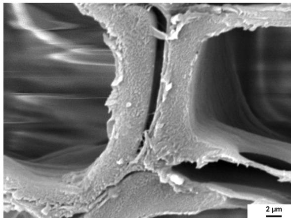
**Figure 5.7.** The SEM micrograph of the cross section of pinewood swelled in acetone – water (MF 0.5)
