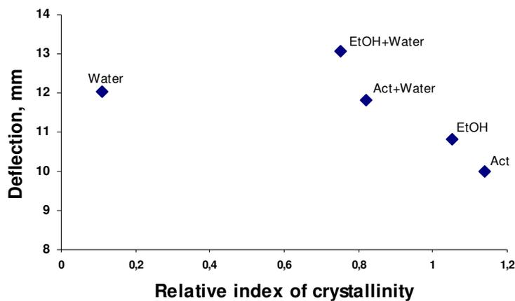
**Figure 5.31.** Relationship between relative index of crystallinity and the deflection.
