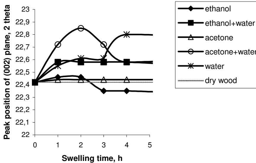
**Figure 5.26.** Shift of the peak position in the (002) plane during swelling of wood in various solutions
