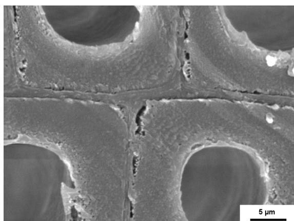
**Figure 5.9.** The SEM micrograph of the cross section of pinewood swelled in the DMF – water (MF 0.5)
