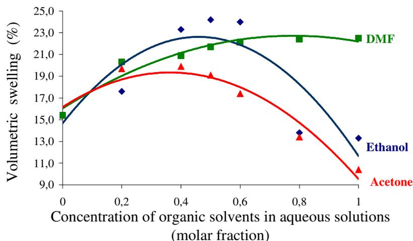
**Figure 5.1.** Volumetric swelling of pinewood in aqueous solutions
