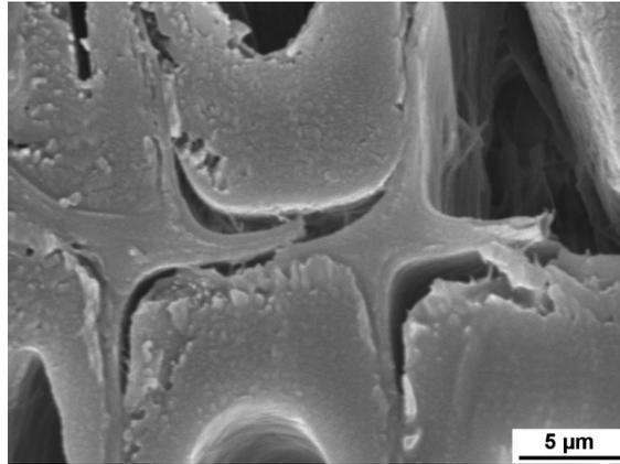
**Figure 5.14.** The SEM micrograph of the cross section of pinewood swelled twice in ethanol (96%)
