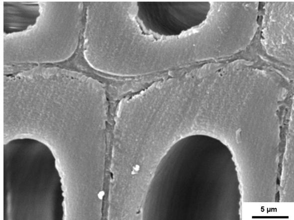
**Figure 5.6.** The SEM micrograph of the cross section of pinewood swelled in acetone
