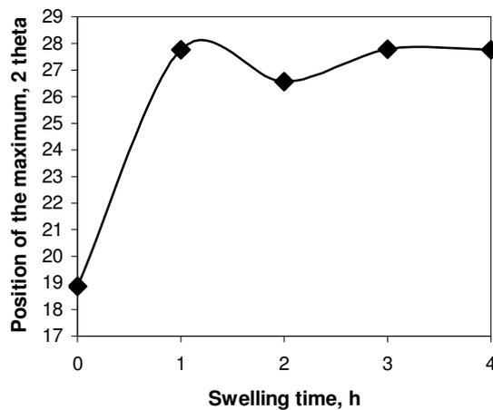
**Figure 5.23.** Dependence of the maximum of the amorphous share of the diffraction pattern of swelled wood (Klason lignin).
