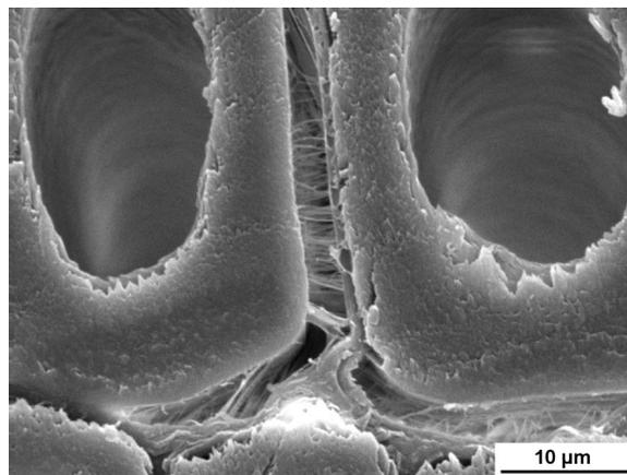
**Figure 5.17.** The SEM micrograph of the cross section of pinewood swelled twice in acetone
