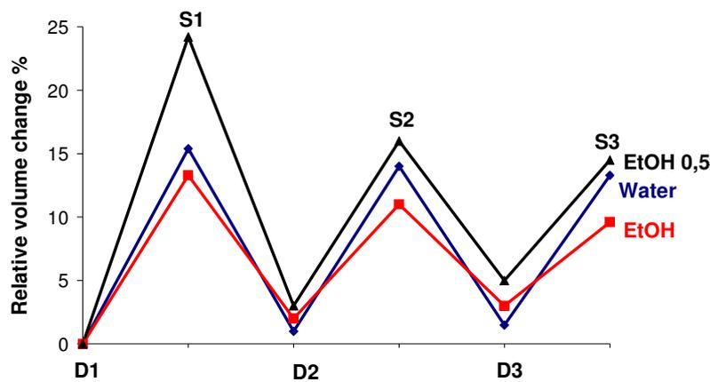
**Figure 5.12.** Cyclic swelling of pinewood in water, ethanol and ethanol aqueous solutions (MF of ethanol 0.5), where S1, S2, S3 are the swelling cycles and D1, D2 and D3 the drying cycles
