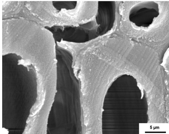
**Figure 5.3.** The SEM micrograph of the cross section of pinewood swelled in ethanol (96%)
