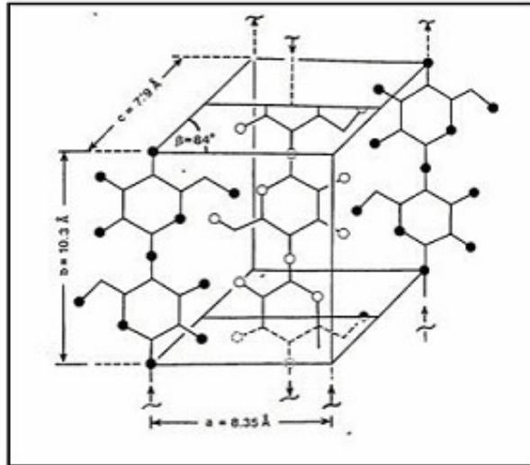
**Figure 5.24.** The structure of a unit cell of cellulose by Meyer and Mischin
