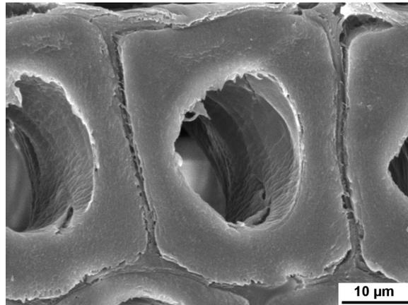
**Figure 5.18.** The SEM micrograph of the cross section of pinewood swelled twice in acetone – water
