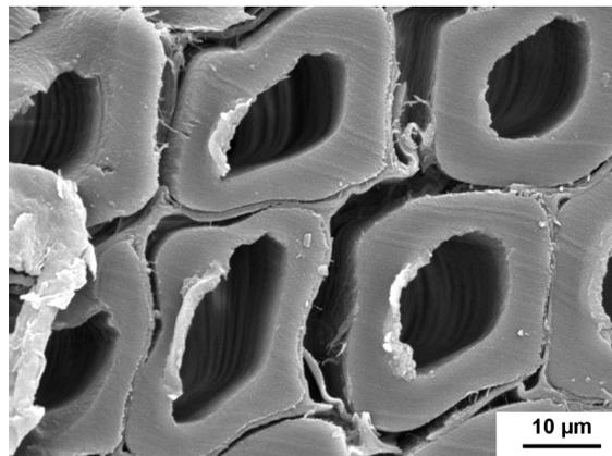
**Figure 5.5.** The SEM micrograph of the cross section of pinewood swelled in ethanol-water (MF 0.5)
