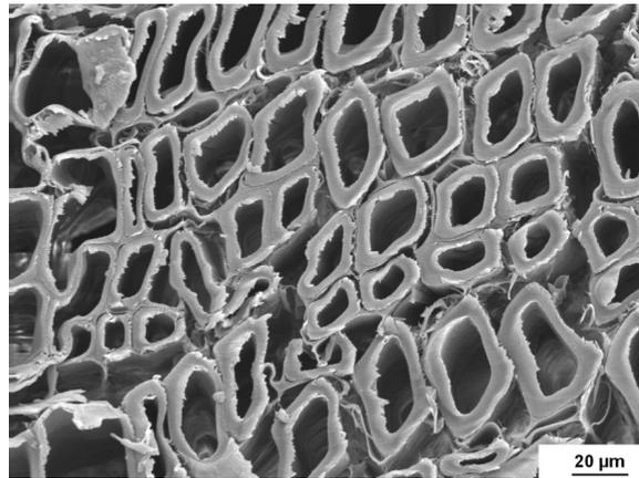
**Figure 5.4.** The SEM micrograph of the cross section of pinewood swelled in ethanol-water (MF 0.5)
