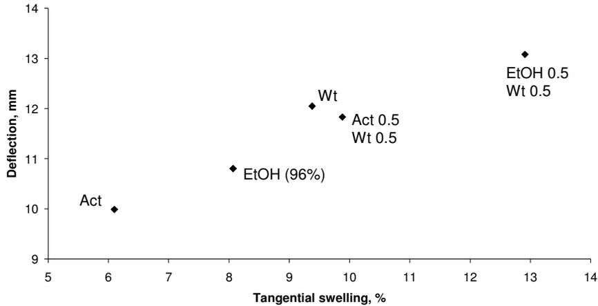
**Figure 5.21.** Deflection as a function of the percentage of tangential swelling and of the liquid
