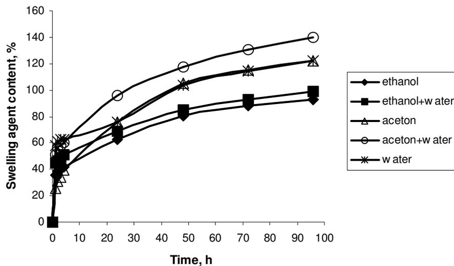
**Figure 5.27.** Relationship between moisture content absorbed into the wood and the swelling time
