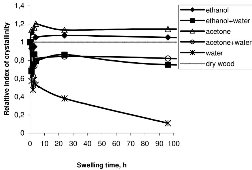
Figure 5.29. Relationship between relative index of crystallinity and the swelling time;
