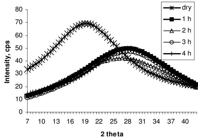
**Figure 5.22.** Drift of the amorphous model compound (Klason lignin) diffraction pattern shape according to the swelling time of the wood sample.
