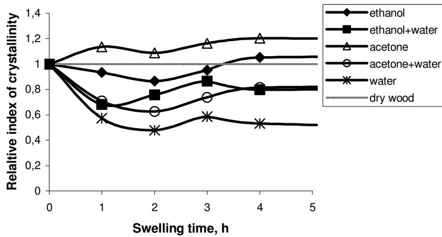
Figure 5.30. Relationship between relative index of crystallinity and the swelling time.
