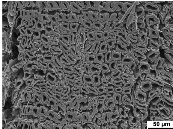
**Figure 5.15.** The SEM micrograph of the cross section of pinewood swelled twice in ethanol – water (MF 0.5)
