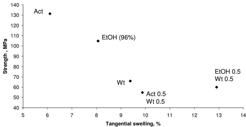
**Figure 5.20.** Bending strength in tangential direction as a function of the percentage of swelling and of the liquid
