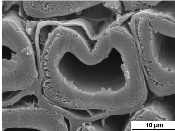
**Figure 5.16.** The SEM micrograph of the cross section of pinewood swelled twice in ethanol – water (MF 0.5)
