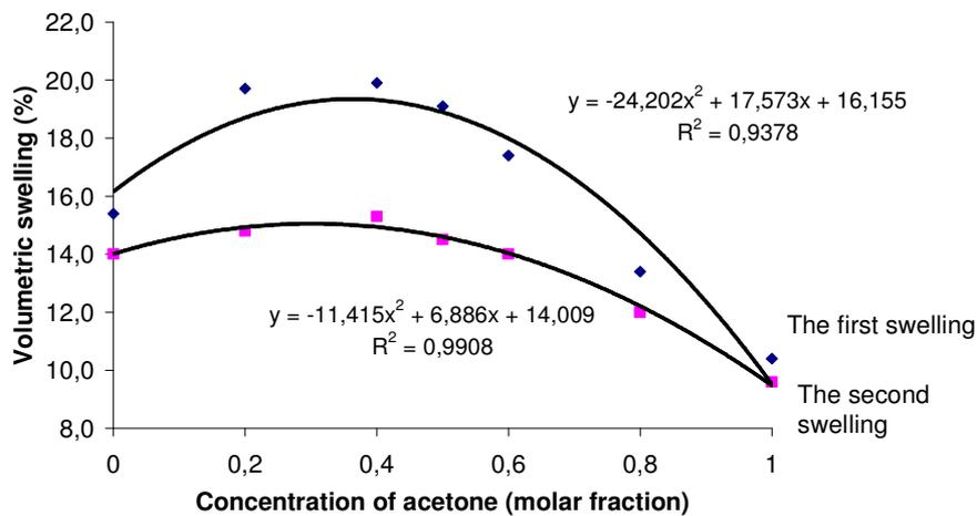
**Figure 5.11.** Repeated swelling of pine sapwood in aqueous solutions of acetone (new solutions)
