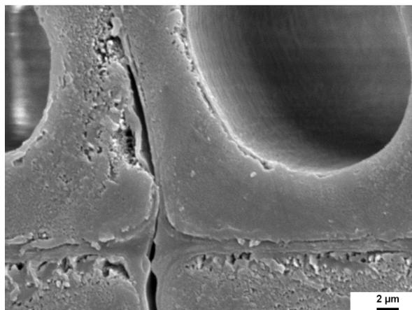
**Figure 5.8.** The SEM micrograph of the cross section of pinewood swelled in DMF
