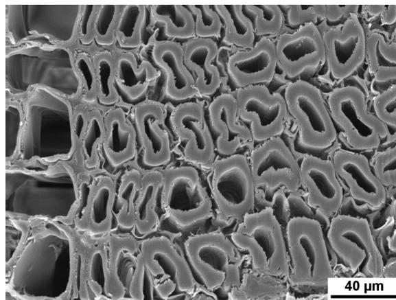
**Figure 5.13.** The SEM micrograph of the cross section of pinewood swelled twice in ethanol (96%)
