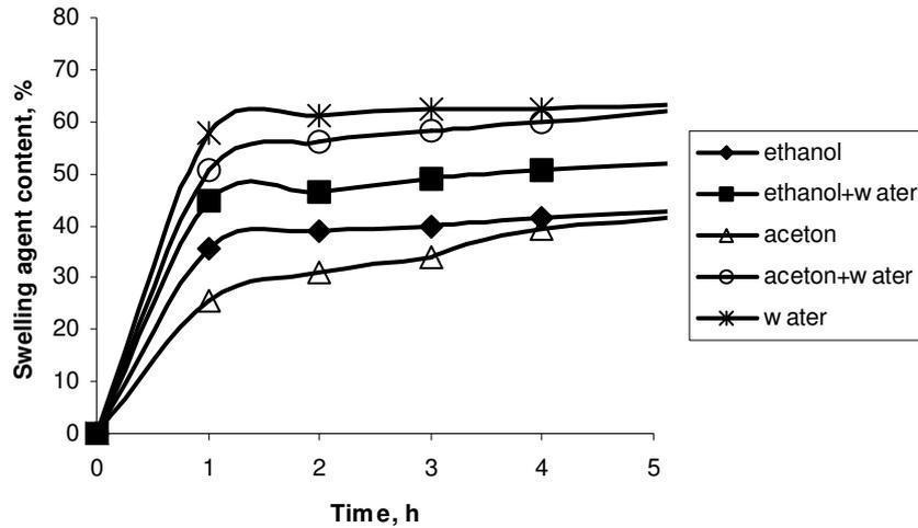
**Figure 5.28.** Relationship between moisture content absorbed into the wood and the swelling time.
