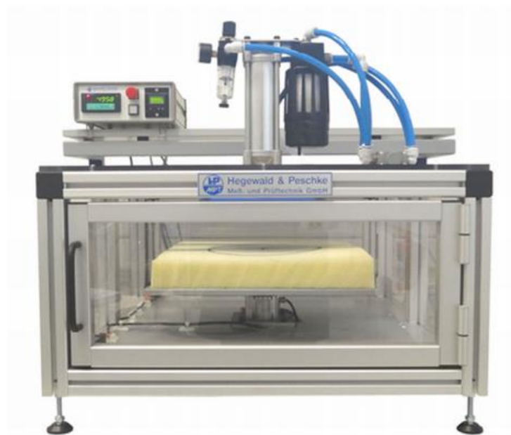
Figure 3.1 Test stand for long-term tests on foamed materials by Hegewald & Peschke
