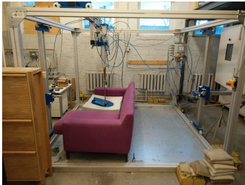
Figure 4.1 Mechanical Hegewald & Peschke furniture test stand
