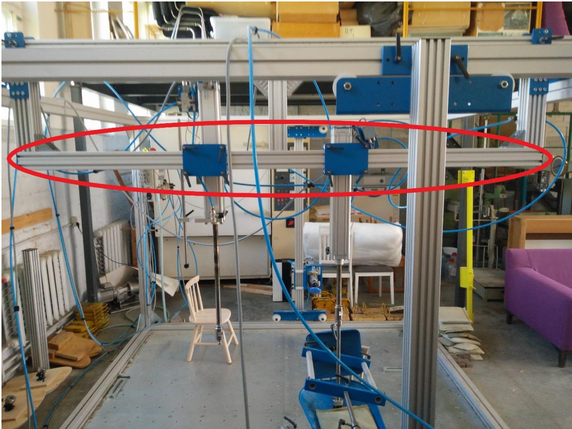
Figure 3.9 Attached profile to existing testing rig (marked with red)
