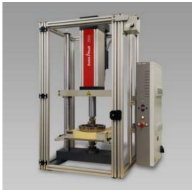
Figure 3.2 Dynamic fatigue test bench 5 kN
