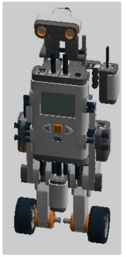
Figure 4.2 design of an inverted pendulum in LDD.
