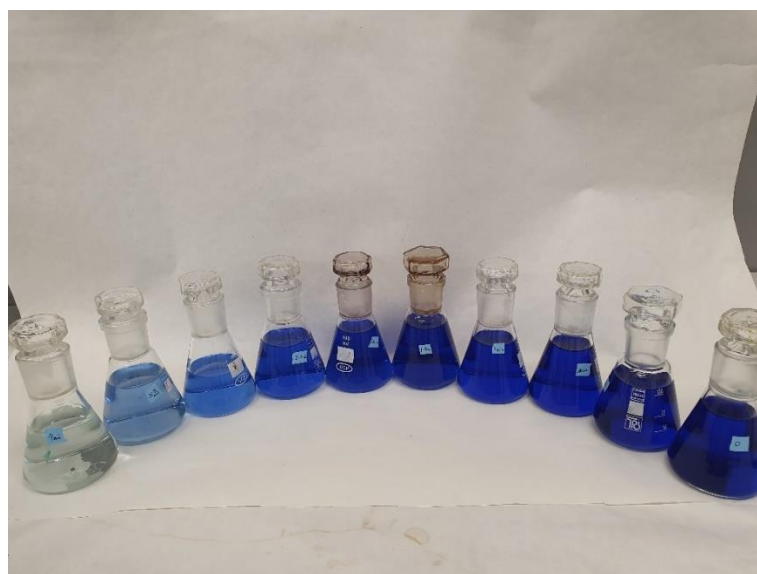
Figure 3.9. Indigo blue dye collected samples at different time intervals from initial state of decolouration to final state: initial concentration, 46mg/L
