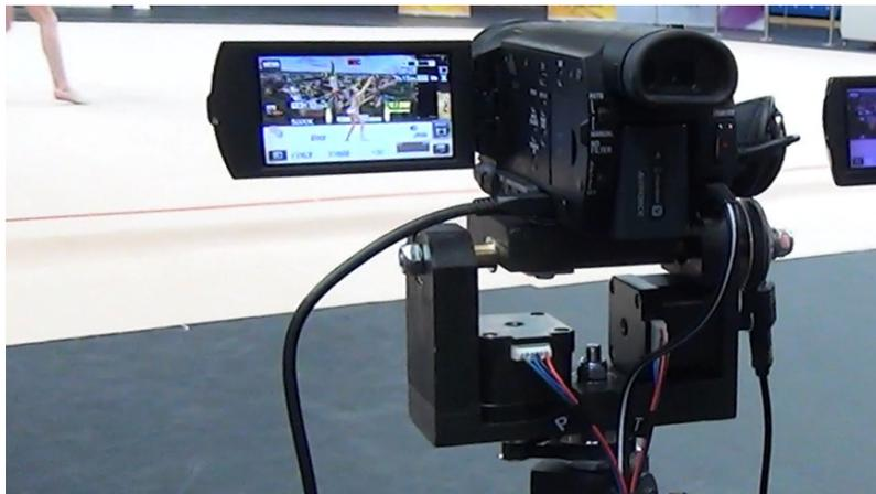
Figure 7. Photo of the assembled pan-tilt head.
