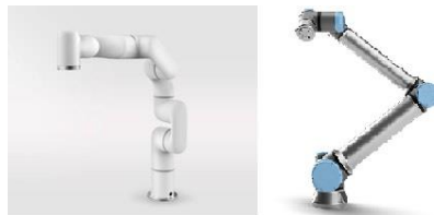
Figure 1.3 4999$ xArm 7 [8] and 56500$ UR10 robot [9]
