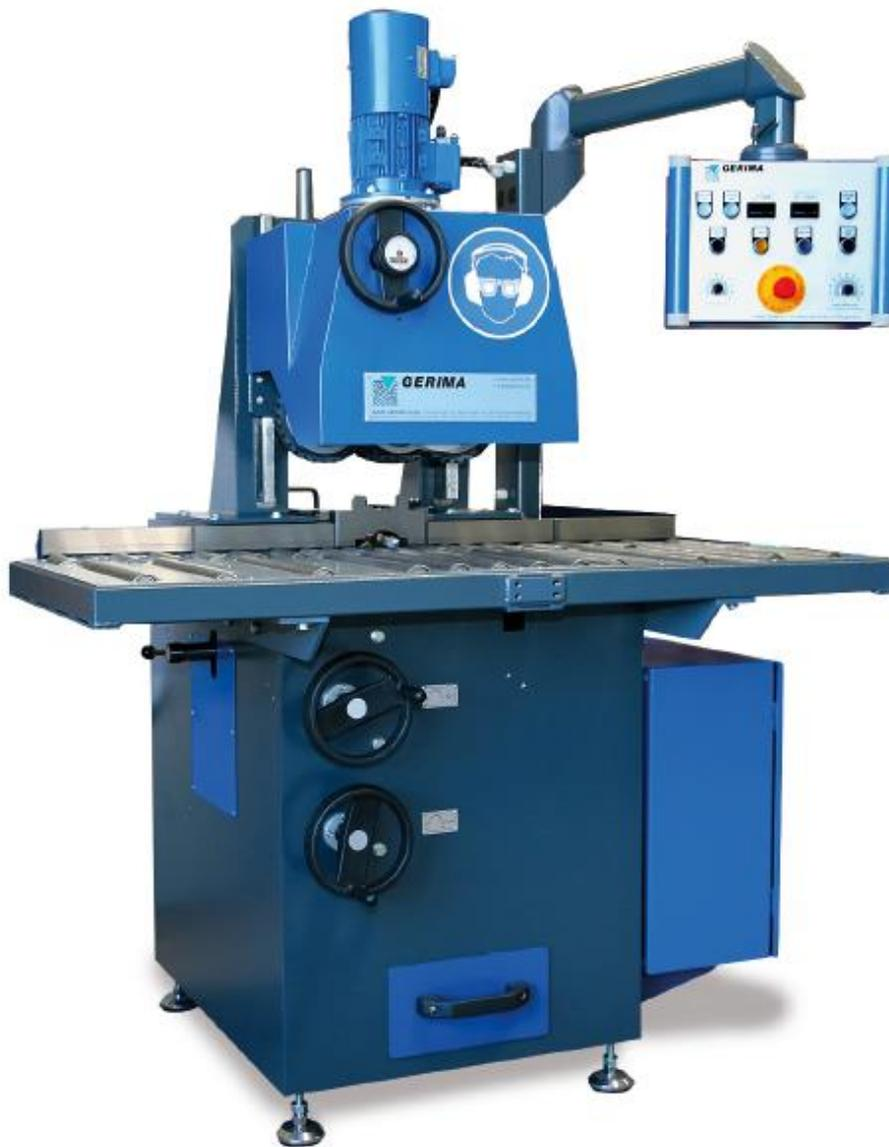
Figure 16 – Stationary beveling machine by MMB600 by GERIMA [15]
