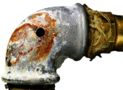
Figure 6 – Destruction caused by corrosion
