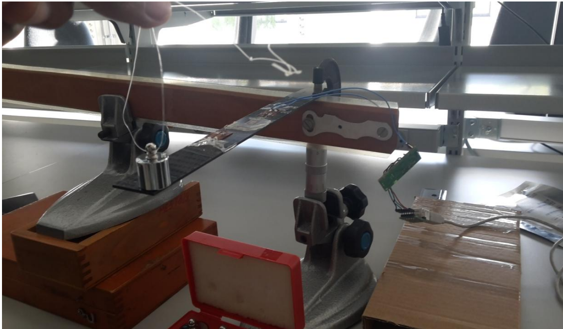
Figure 33. Force Sensor Module Laboratory Test Setup
