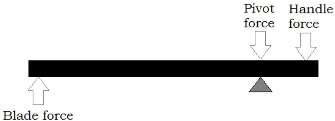
Figure 30. The Forces Present on a Paddle
