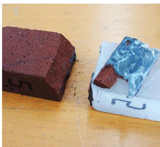
**Figure 69.** Disjointed adhesive layer (F)
