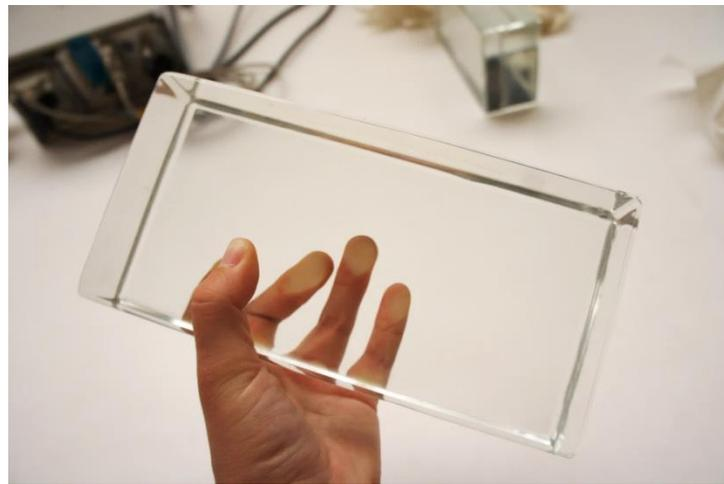
**Figure 34.** Low-iron completely transparent soda-lime glass block
