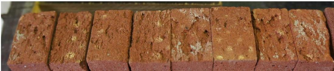
**Figure 62.** Medium rough (salt on surface)
