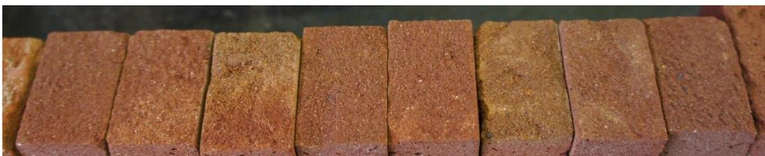
**Figure 63.** Rough (loose particles on surface)
