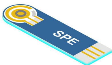
Figure 1.3 Tools for electrochemical detection on SPE sensors. (a) a SPE sensor chip, (b) a portable wireless potentiostat [66]
