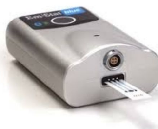
Figure 1.3 Tools for electrochemical detection on SPE sensors. (a) a SPE sensor chip, (b) a portable wireless potentiostat [66]
