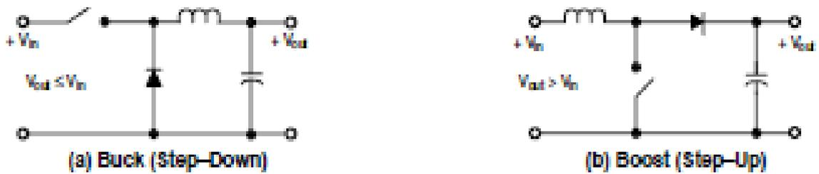
Fig 1.7 Two basic switching voltage regulators
