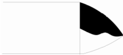
Figure 8 Two pahases in Tylor cone (on the Figure the black part presents the carbon black and the white part is the PVA in water / alcohol)
