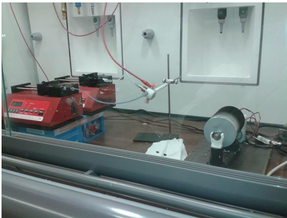
Figure 4 Coaxial electrospinning setup
