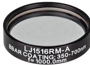
**Figure 7:** Plano-convex cylindrical lens, LJ1516RM-A, by Thorlabs. Focal length of  $f = 1000$  mm, diameter of 1 inch and made out of light transmissible borosilicate-crown glass material - N-BK7.
