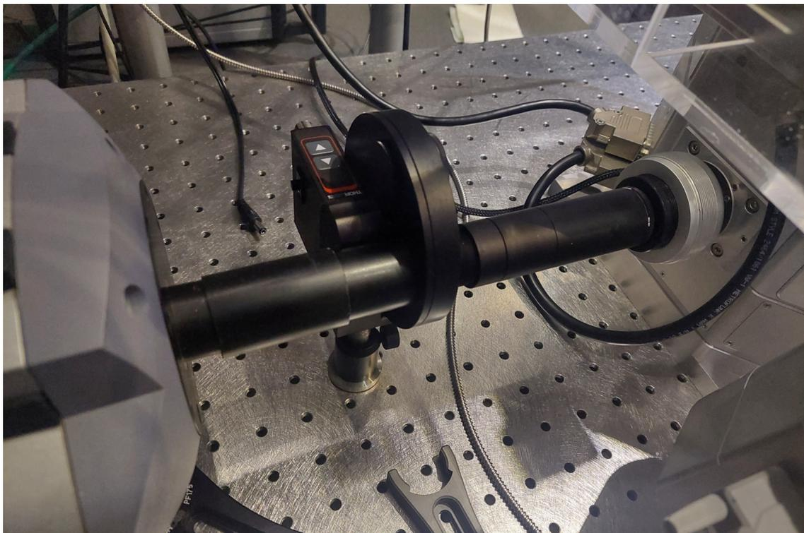
**Figure 8:** Filter wheel connected to the camera and microscope housing with lens tubes.
