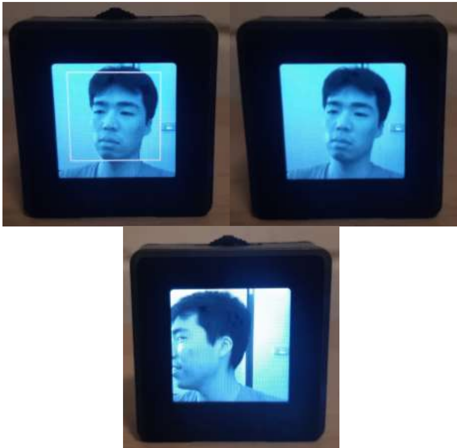
Figure 4.3 Frontal face recognized(left), frontal face not recognized (right), side face not recognized (middle)
