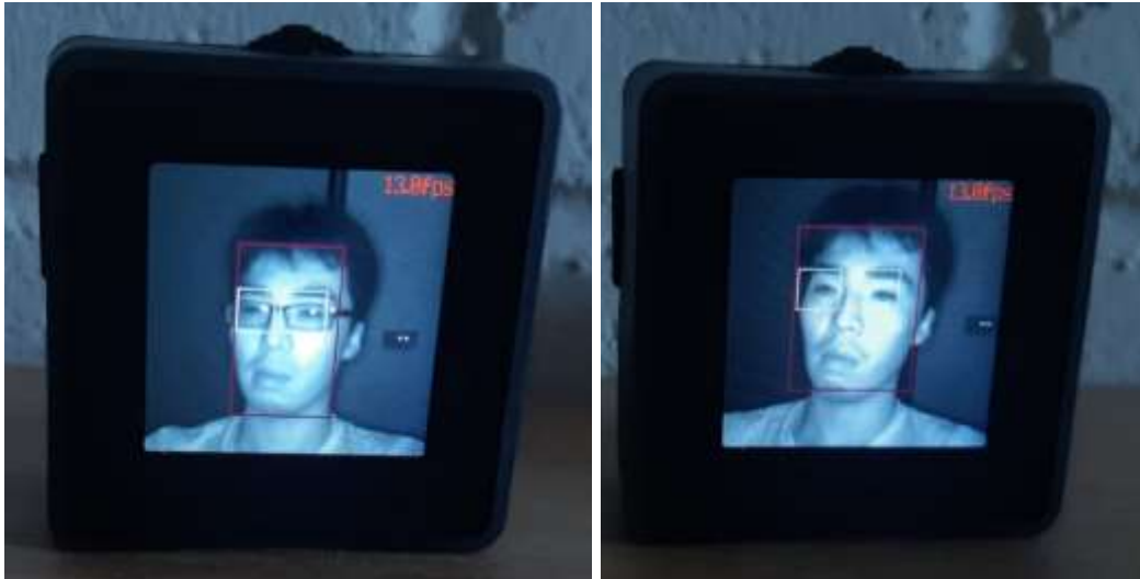
Figure 4.10 Model results on night conditions, without glasses (left) and with glasses (right).
