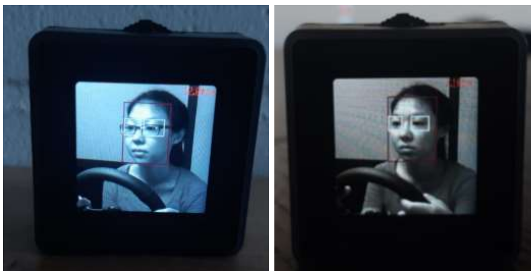
Figure 4.9 Model results on daytime conditions, with glasses (left) and without glasses (right)
