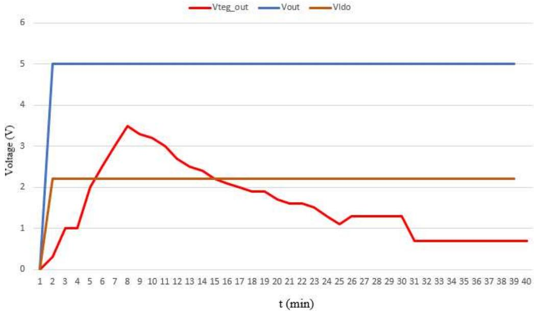
Figure 27: DC converter output graph for TEG elements connected in series. The TEG output is represented with the red line and labelled as  $V_{teg\_out}$ , DC converter  $V_{out}$  is represented with the blue line (labelled as  $V_{out}$ ) and  $V_{LDO}$  output of DC converter is represented with the brown line (labelled  $V_{ldo}$ ).
