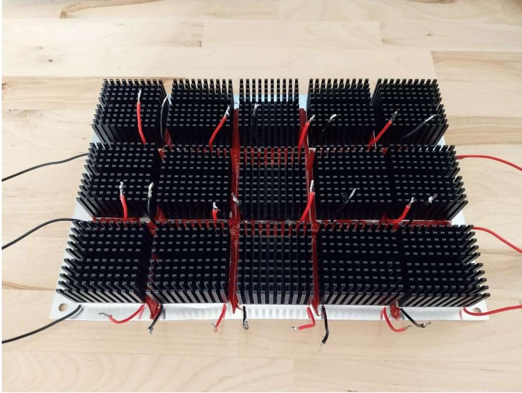
Figure 10: Photograph of the initial developed prototype TEG assembly with 15 Peltier elements for the proposed TEG. Notice that the elements are not connected, which allows testing different configurations of series and parallel connections.
