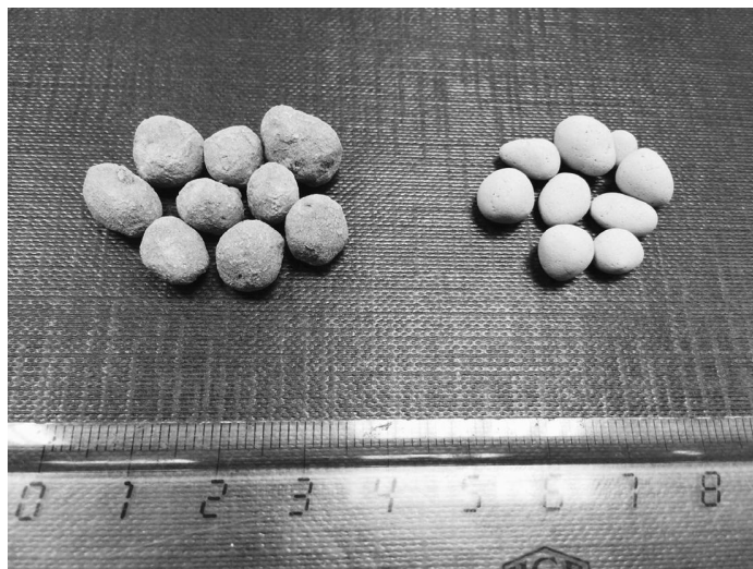
Fig. 9. The granules before and after the leaching test.
