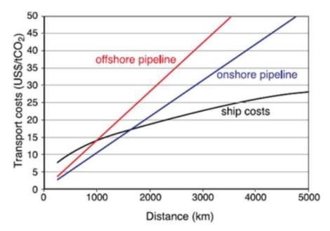
Figure 1.2 Approximate cost comparison of  $CO_2$  transportation with offshore pipeline, onshore pipeline and ship [9]
