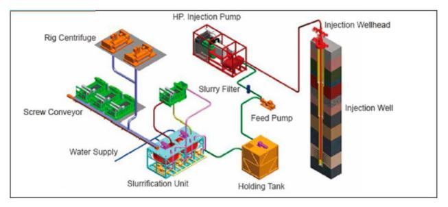
Figure A 1.1 CRI operation sequence and components. Source: http://go.jereh.com/Product/CRI-16S-Waste-Injection-Technology-And-Package-Unit-339.html
