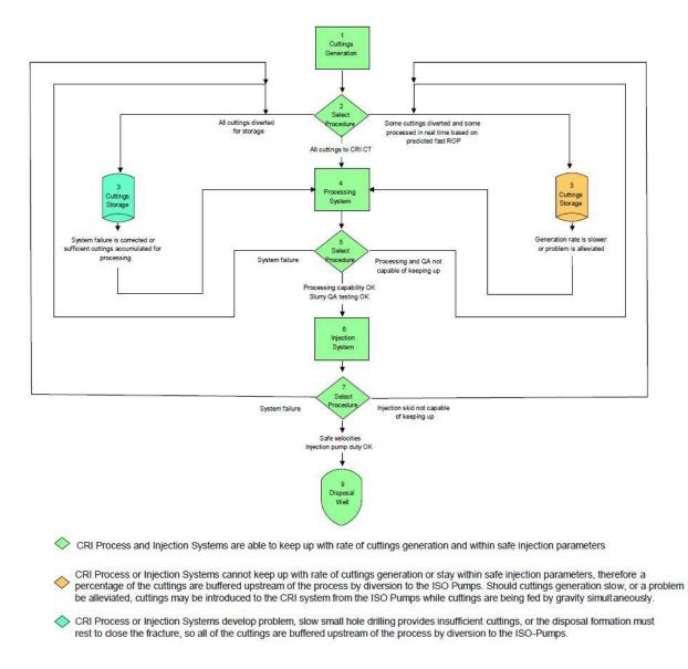
Figure 2.5 Basic-Flow-Path schematic diagram [24].
