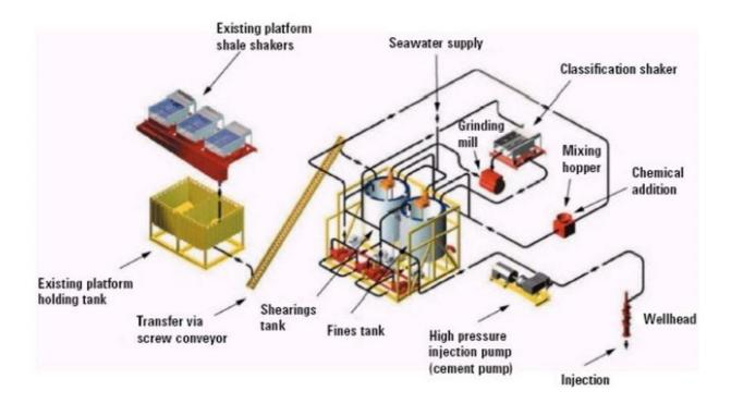
Figure 2.4 Schematic of cuttings re-injection system [25]
