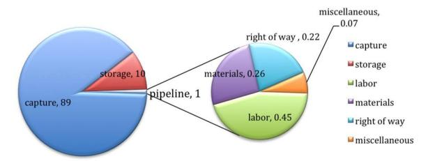
Figure 2.7 Breakdown of CCS project costs and CO<sub>2</sub> pipeline cost [26]
