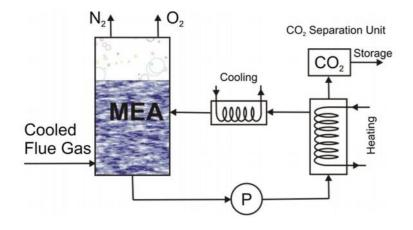
**Figure A 2.1 Mono ethanolomine scrubbing process. Source:** Advanced CO<sub>2</sub> Capture Process Using MEA Scrubbing: Configuration of a Split Flow and Phase Separation Heat Exchanger
