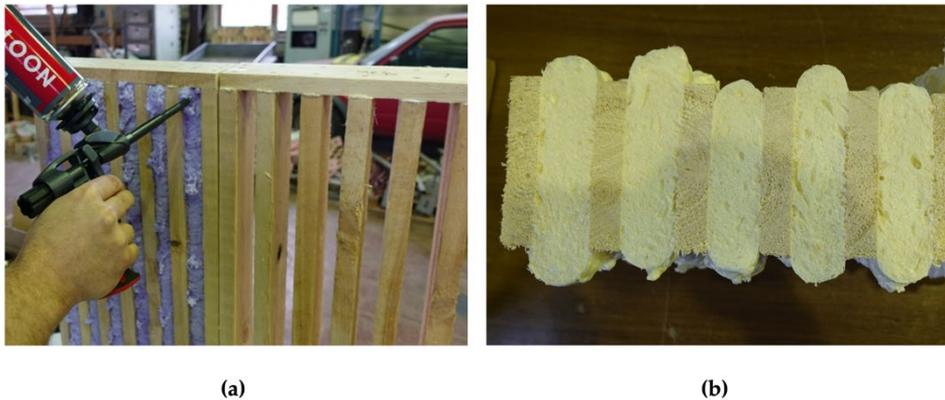
Figure 5. Filling the joints in a wooden frame (a) and an example of the cross section (from above) of the frame with filled joints (b).
