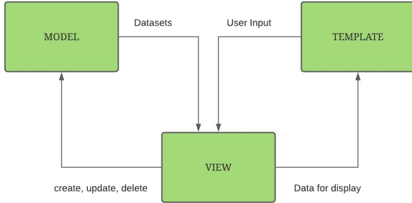
Figure 14. Data processing structure using Django framework
